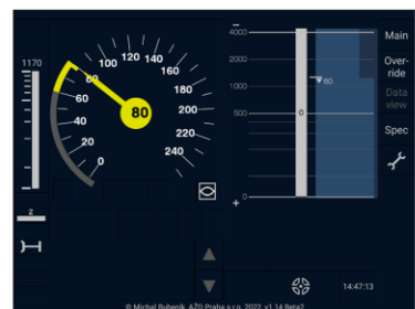
Freight train, 673 m, braked in P mode, 87 BWP; SB in TSM allowed
