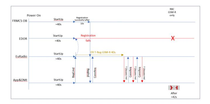
Figure 6 No GSM-R, FRMCS available, GSM-R only RBC <An additional "adapter lane" should be added to the Figure. It needs to be checked whether the radio connection failure symbol appears also in the adapter case.>
