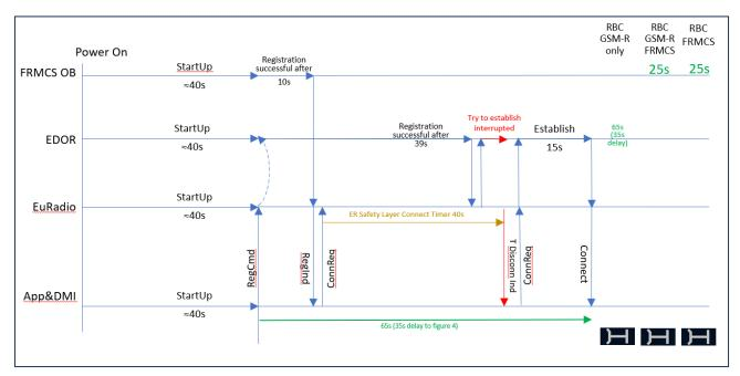
Figure 5 GSM-R / FRMCS available, but GSM-R registration late <a href="#">An additional "adapter lane" should be added to the Figure</a>>
