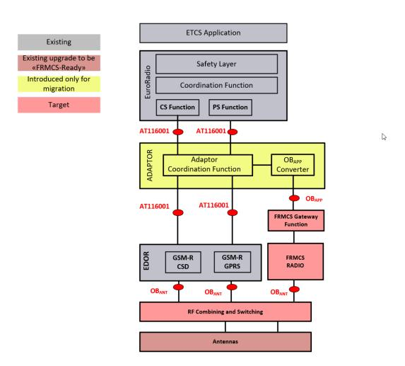
Figure 2 On-board logical architecture
