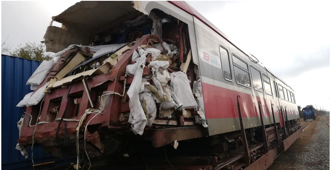
Figure 3.4.4.2: External appearance of the driver cab of the motor wagon 711-078 DMV 711-077/078 at the train No. 25412 after the serious accident
