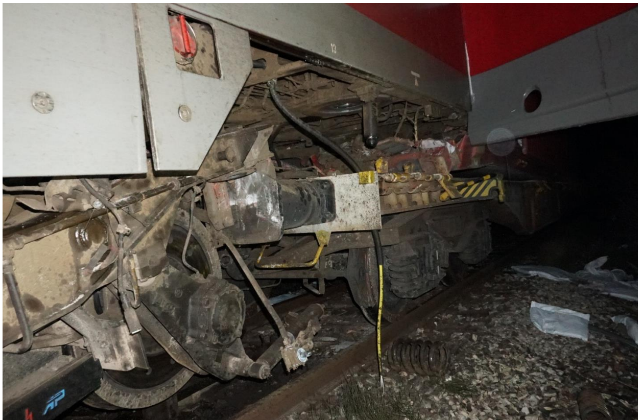
Figure 4.1.3: Appearance of the damages on the wagon No. 33 68 4952 037-2
