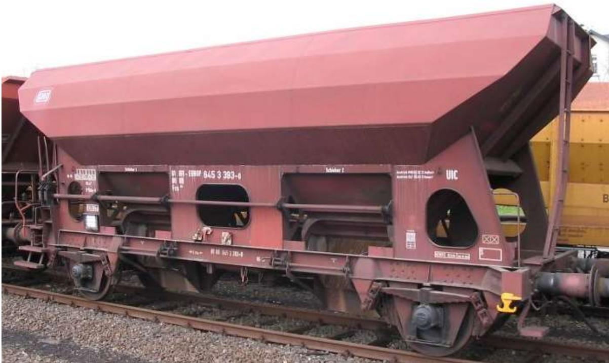
Figure 3 - Example of a unit consisting of a (freight) wagon that can be operated separately, featuring an individual frame mounted on its own set of wheels
