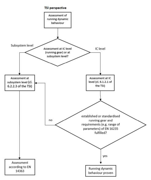
Figure 9 – Flow chart of all the possibilities to prove the running dynamic behaviour in the TSI
