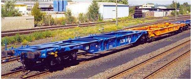
Figure 4 - Example 1 of a unit consisting of a rake of permanently connected two elements (blue and orange), those elements cannot be operated separately (articulated wagon)
