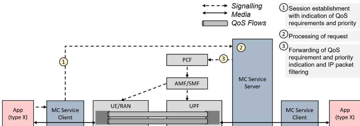
Figure 14-2: 3GPP QoS signalling relevant for interoperability
