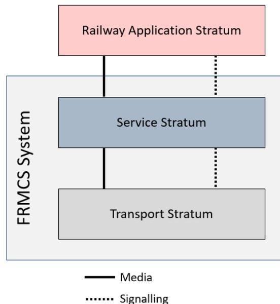
Figure 5-1 Railway Application, Service and Transport Strata
