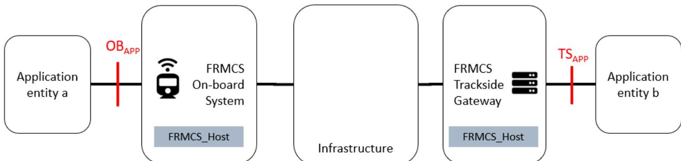
Figure 6-10: Host-to-Host (H2H) addressing principle (Loose-coupled example)
