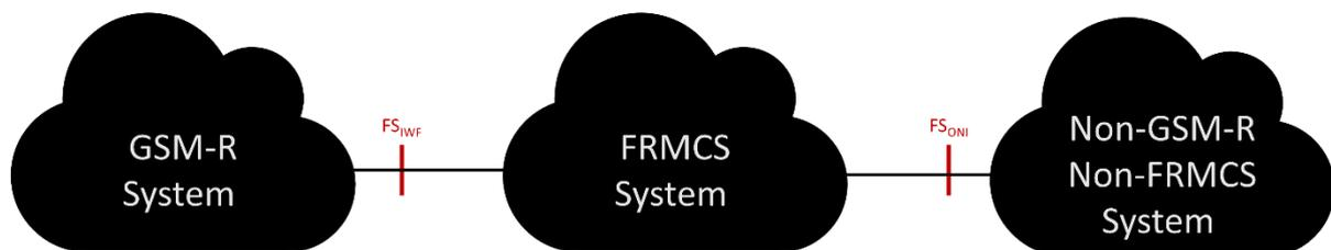
Figure 6-9 - FRMCS System: reference points towards external systems
