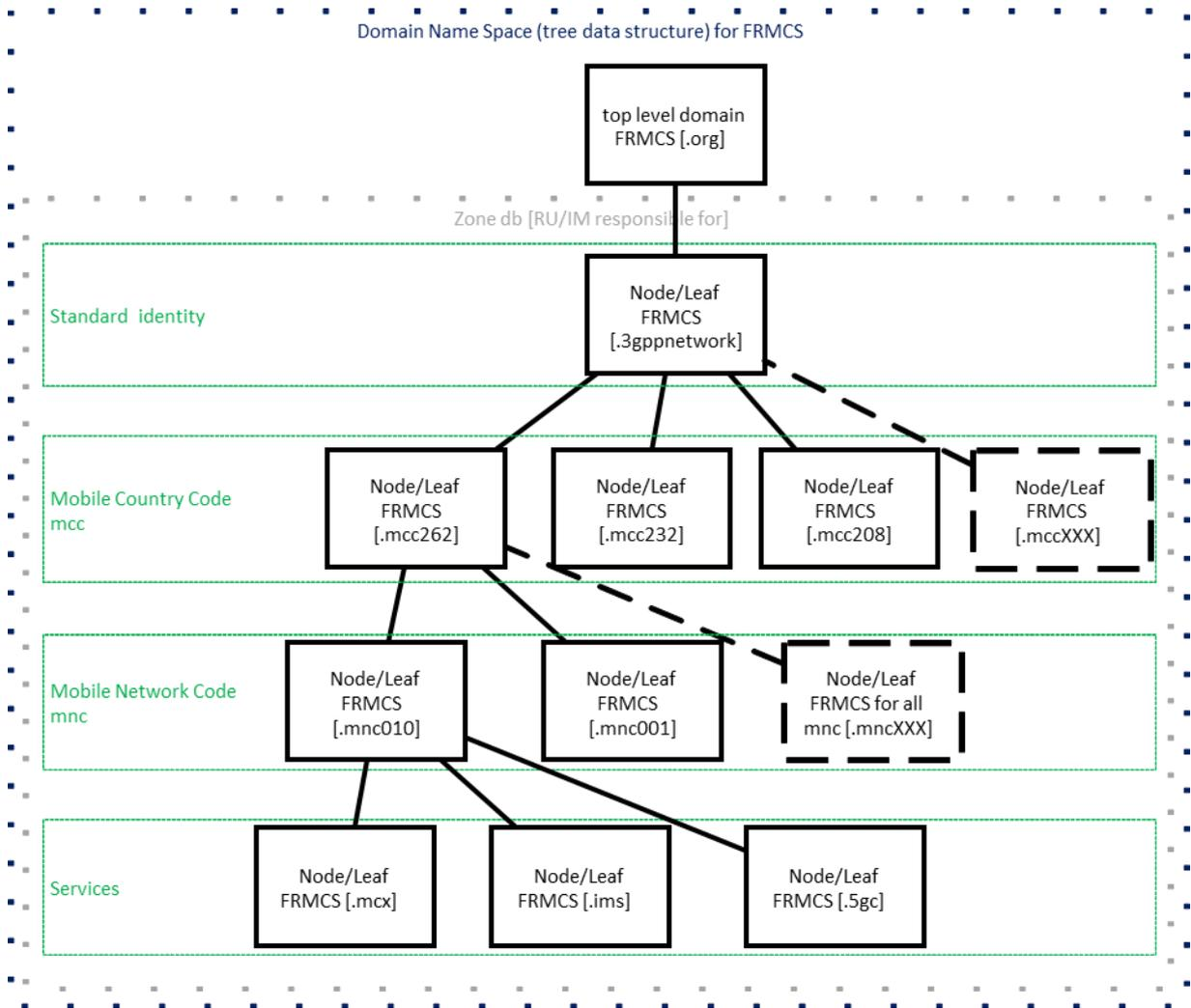
Figure 11-3: Domain Name Space for FRMCS (machine-type communication)
