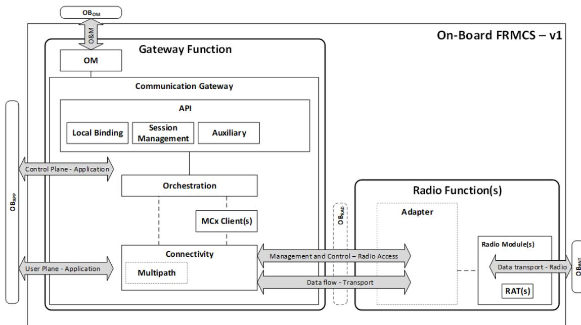
Figure 7-2: On-Board FRMCS architecture
