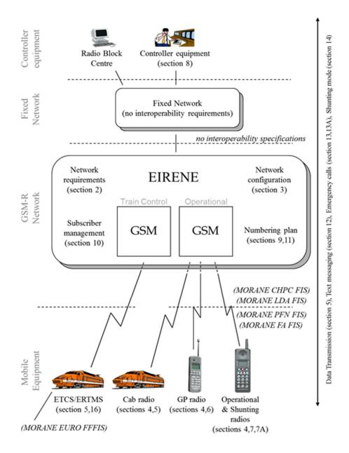
Figure 1-1: Layout of EIRENE specifications and details of interfaces
