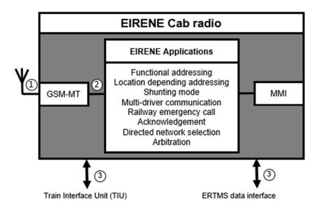
Figure 5-1: Logical Cab radio architecture and interfaces
