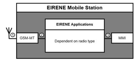
Figure 4-1: Logical mobile radio architecture and interfaces
