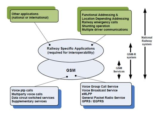
Figure 1-2: Scope of the GSM-R system with reference to functionality provided by GSM
