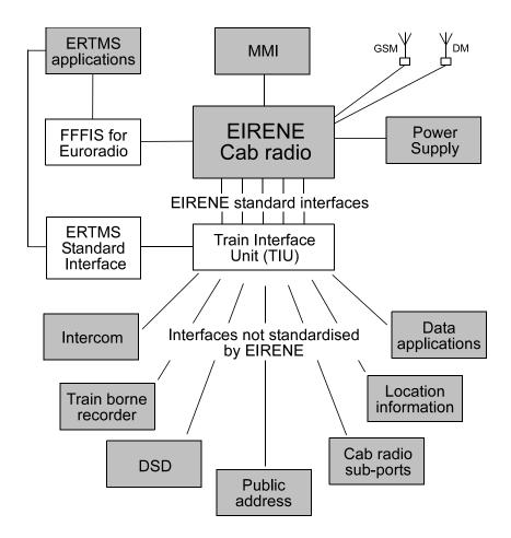
Figure 5-3: Interfaces to the Cab radio
