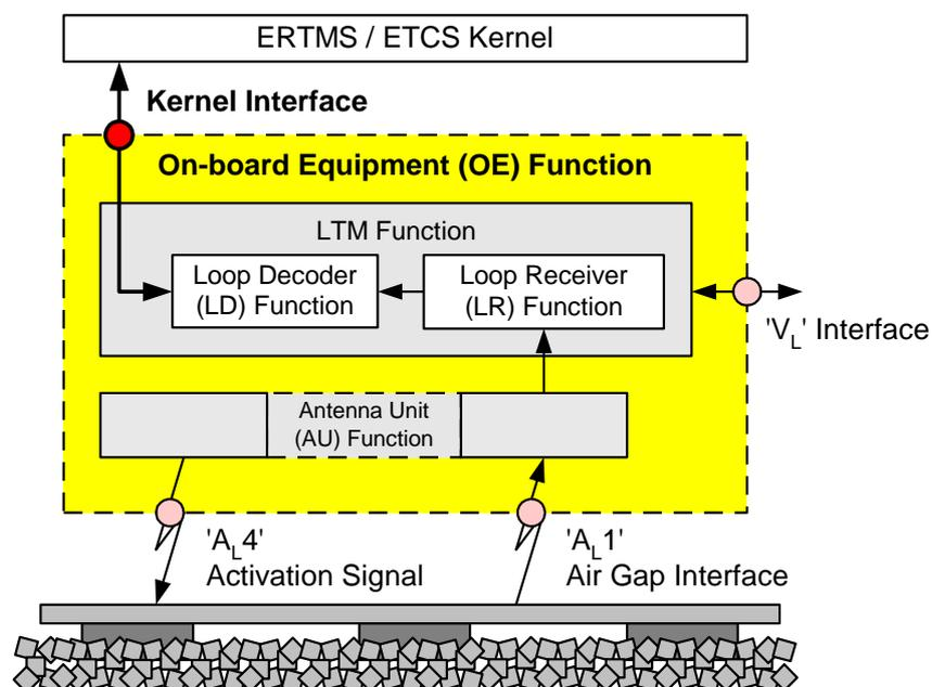
Figure 7-4: Kernel Interface of On-board Equipment
