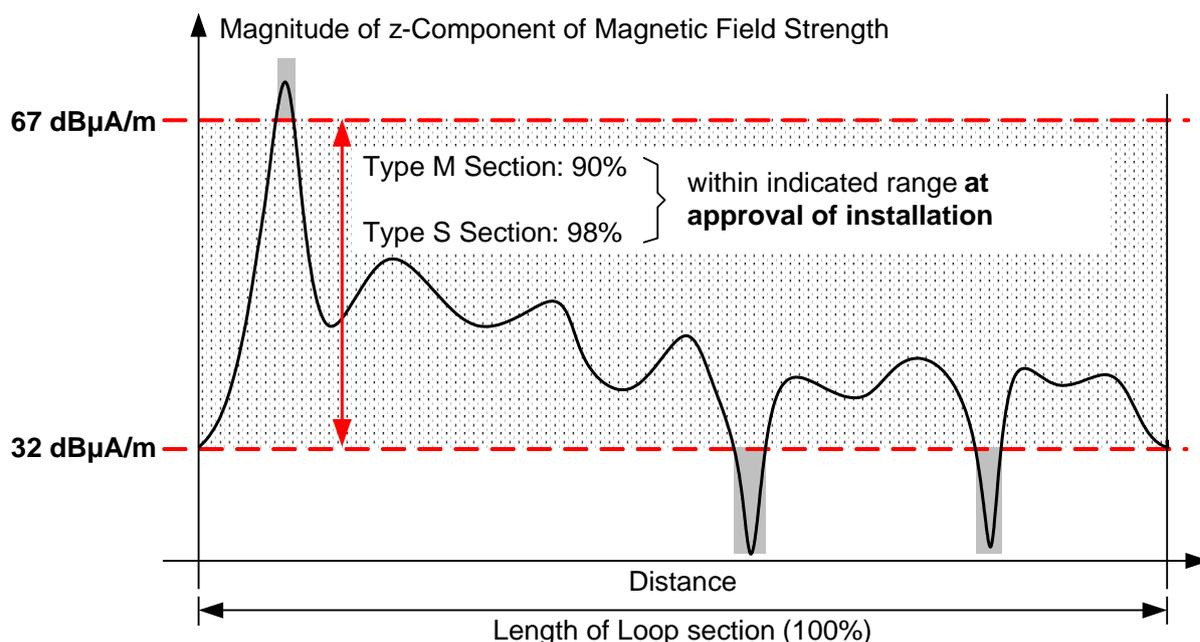
**Figure 6-22: Limits on the Magnitude of z-Component of Magnetic Field Strength in the Air Gap at the Reference Position for Loop Sections of Type M and S**
