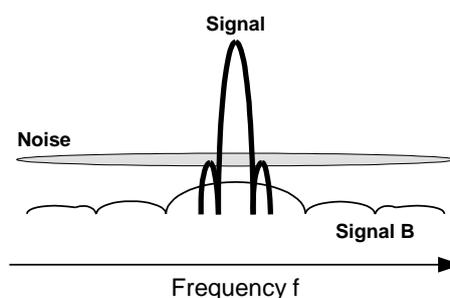
**Figure B- 3: Spectral Behaviour of CDMA Signals**
