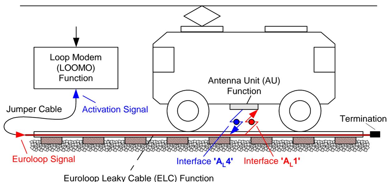
Figure 6-18: Air Gap Interfaces 'A<sub>L4</sub>' and 'A<sub>L1</sub>'
