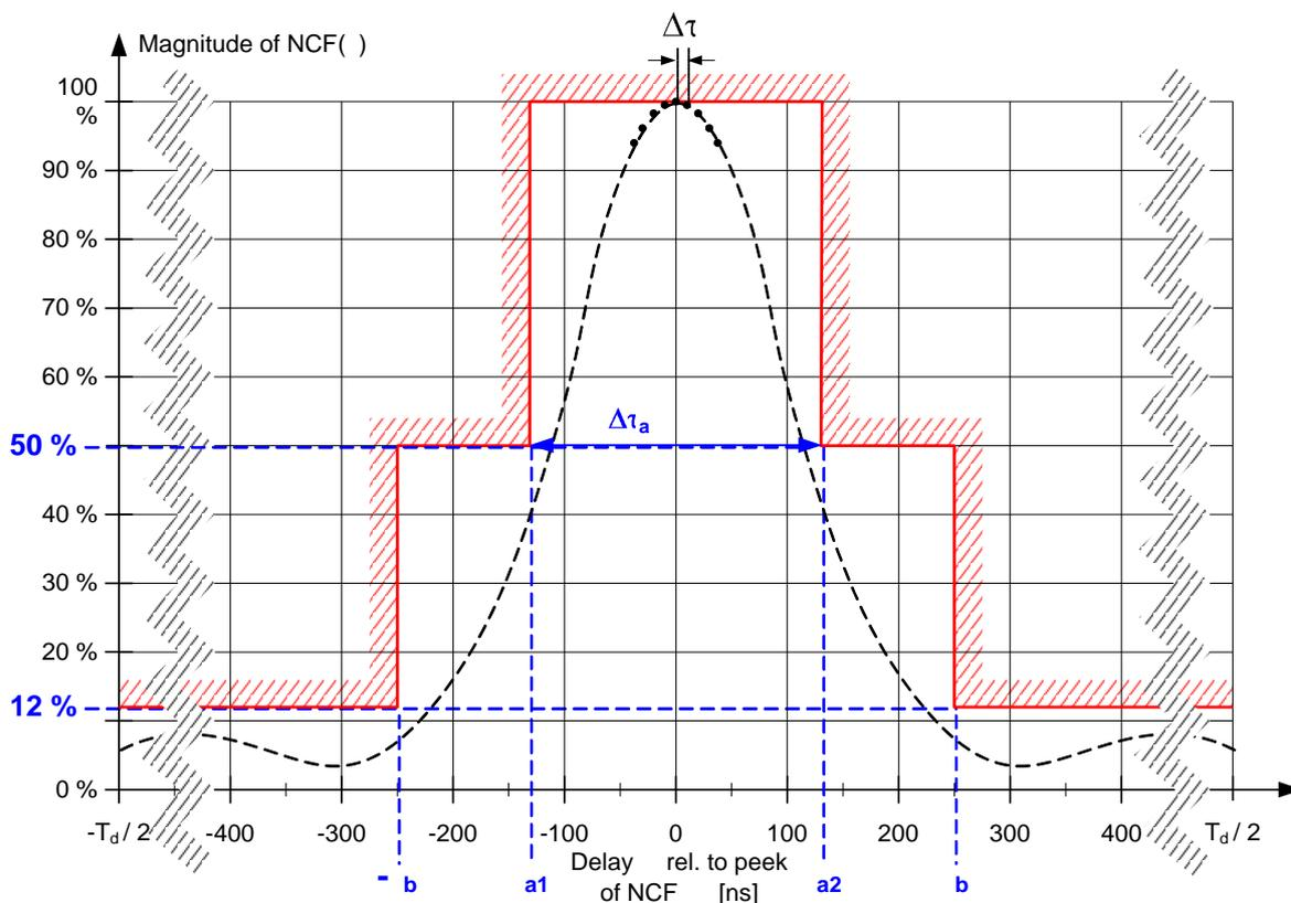
**Figure 6-16: Mask for the Normalised Correlation Function NCF(τ)**
