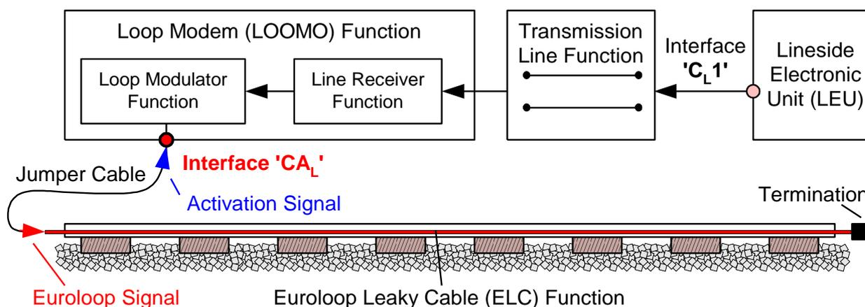
Figure 6-11: Signal Transmission between LOOMO and ELC
