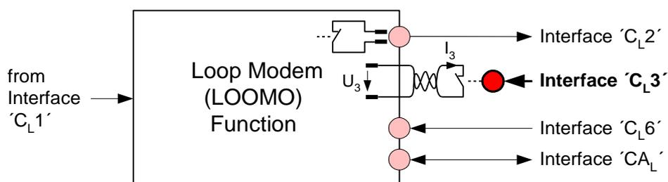
**Figure 6-9: External Activation Interface 'C<sub>L3</sub>' of LOOMO**
