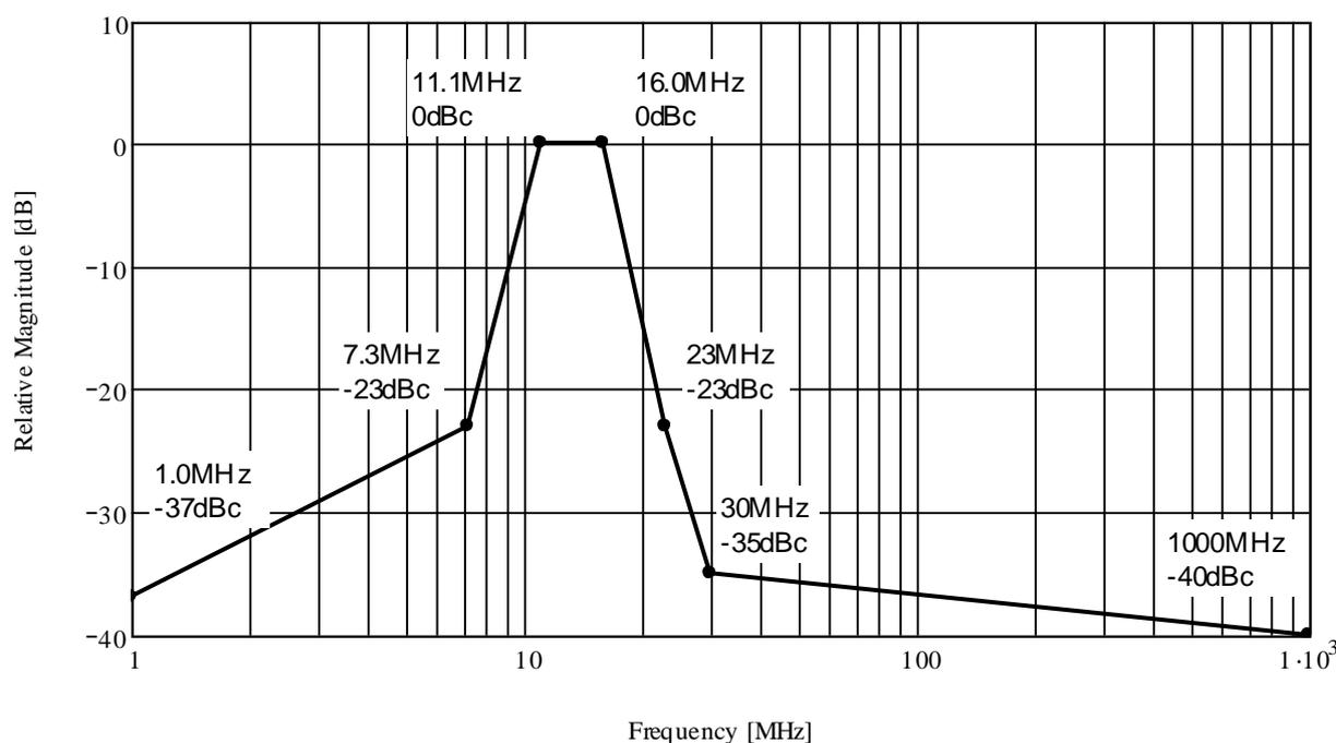
Figure 6-17: Spectrum Mask of Euroloop Up-link Signal
