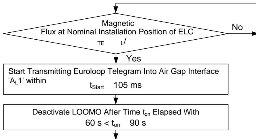
**Figure 6-19: Flow Diagram for Activation of LOOMO by Activation Signal from Interface 'A<sub>L4</sub>'**
