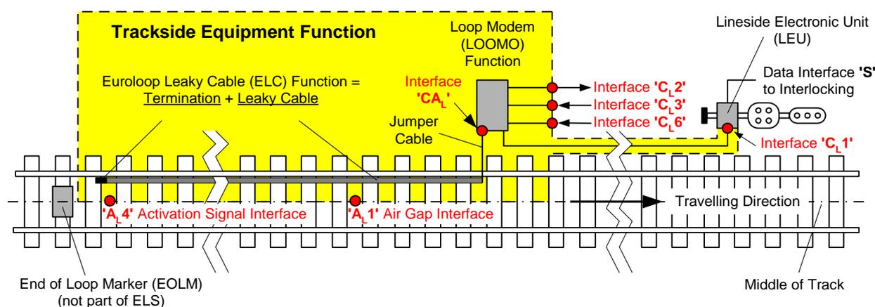
**Figure 6-1: Trackside Equipment of Euroloop Subsystem (unidirectional installation)**
