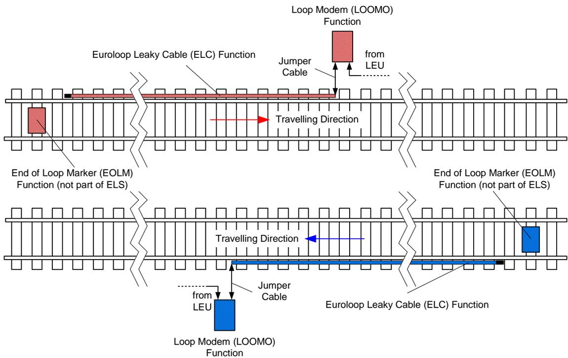
**Figure 6-4: Possible Realisation of a Parallel Euroloop Arrangement**
