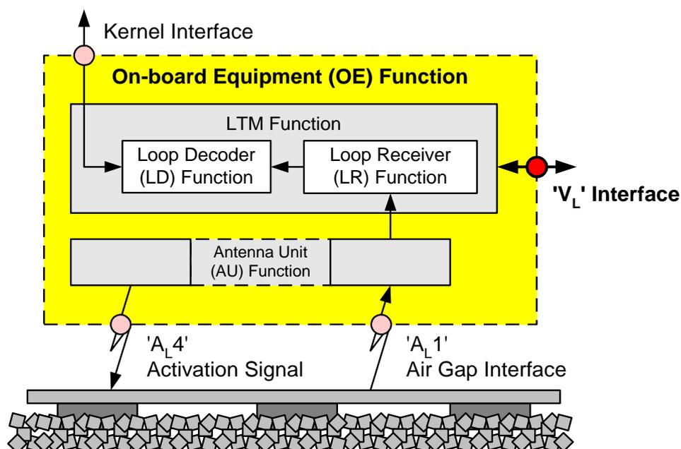
Figure 7-5: Interface 'V<sub>L</sub>' of On-board Equipment
