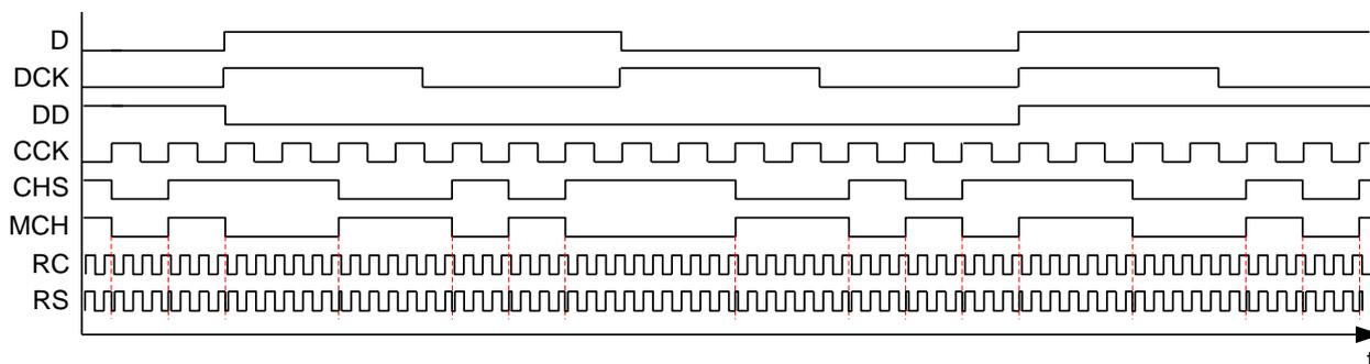
**Figure 6-13: Signals Associated with DSSS Modulation (Informative)**
