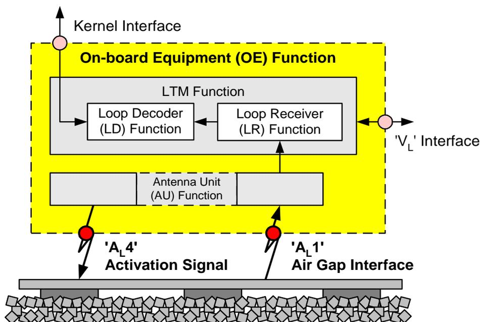
Figure 7-2: Air Gap Interfaces of On-board Equipment
