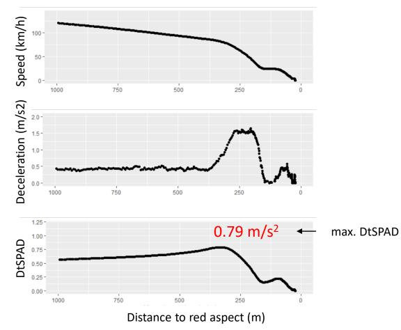
\*mDtSPAD = maximum Dececleration to SPAD, or the maximum required deceleration to to stop in front of the aspect (per approach)
