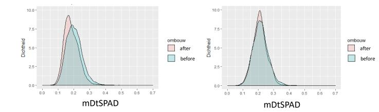
\*mDtSPAD = maximum Dececleration to SPAD, or the maximum required deceleration to to stop in front of the aspect (per approach)
