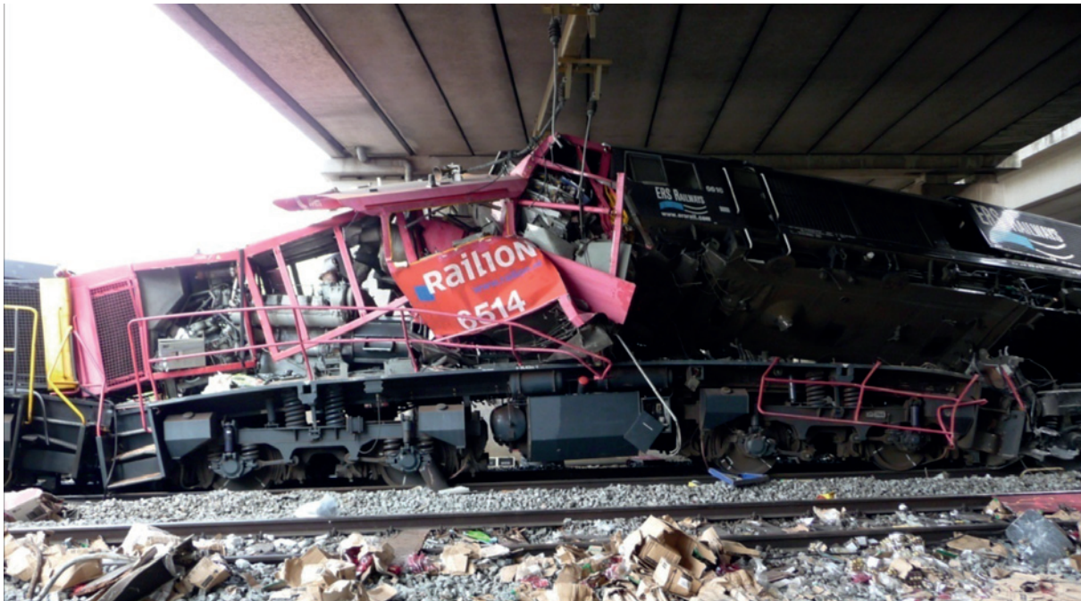
Figure 5: The damage to the locomotives of the two goods trains (in daylight)
