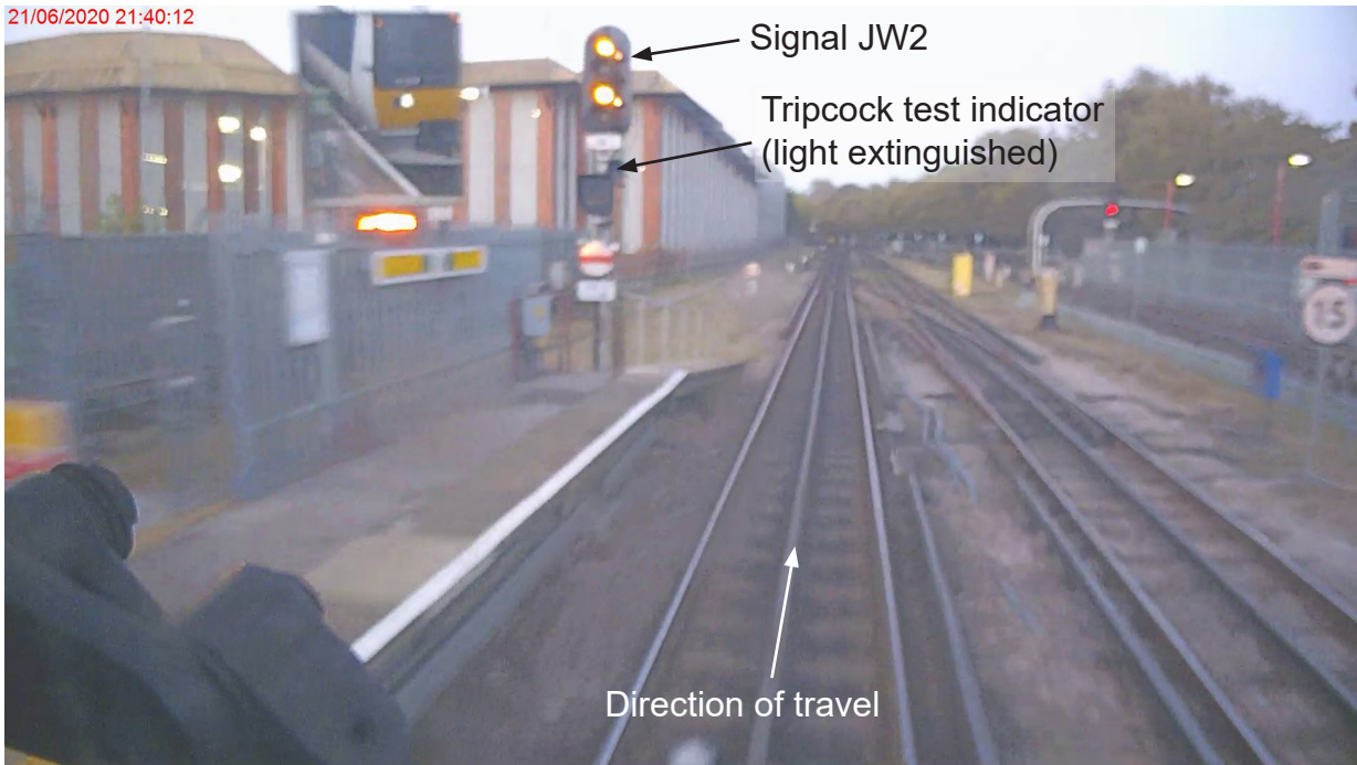
Figure 7: Signal JW2 displaying a double yellow aspect (FFCCTV image courtesy of Chiltern Railways)
