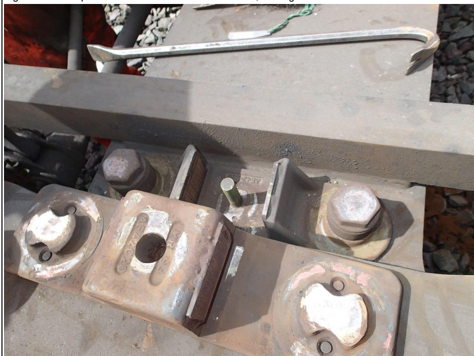
Figure 3: Sidebearer showing signs of frequent contact with end stops
