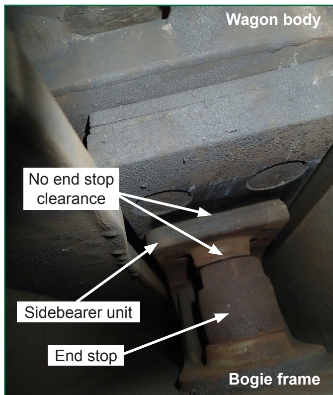
Figure 13: Sidebearer on the left side of the bogie which derailed, showing no clearance between sidebearer casting and end stop (arrowed)
