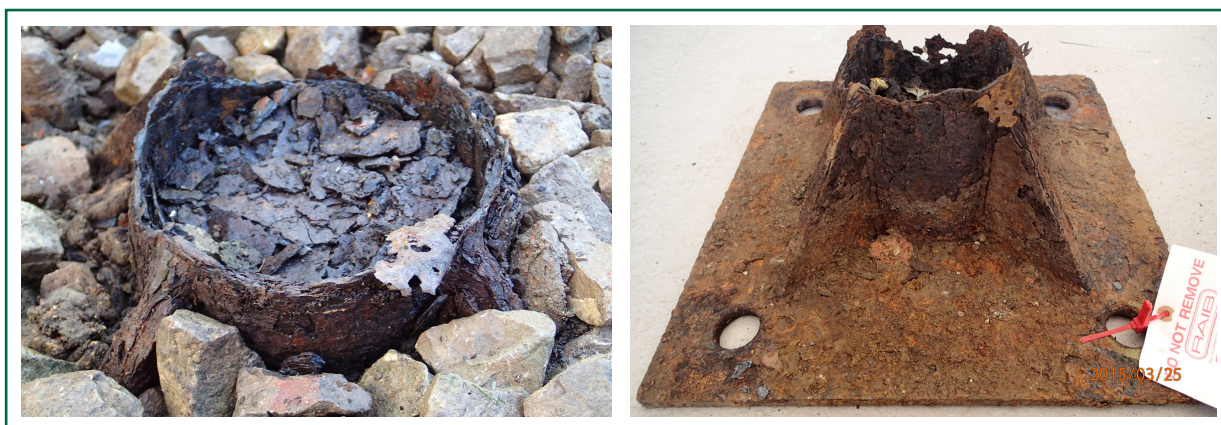
Figure 8: Corrosion at the baseplate (a) in situ after the accident (left image; note level of ballast) and (b) after removal from site
