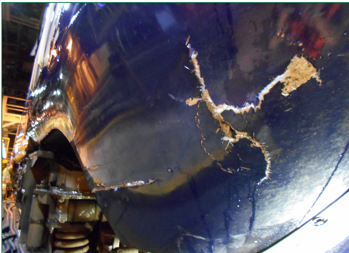
Figure 4: Damage to power car 43160 (courtesy of First Greater Western)
