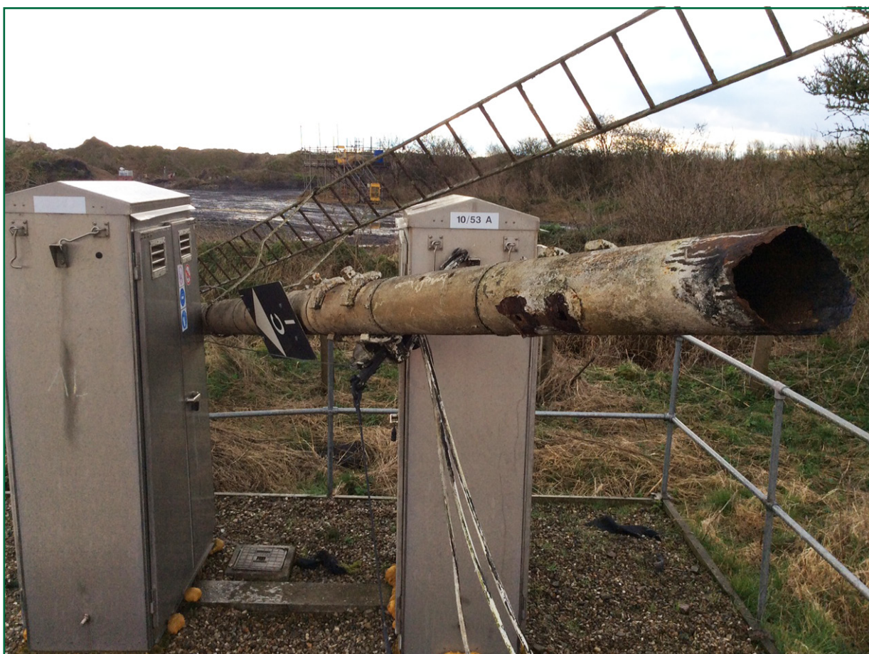
Figure 15: Photograph of the failed signal post at Cantley (courtesy of Network Rail)
