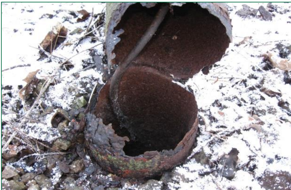
Figure 14: Photograph of the failed signal post at Wymondham (courtesy of Network Rail)
