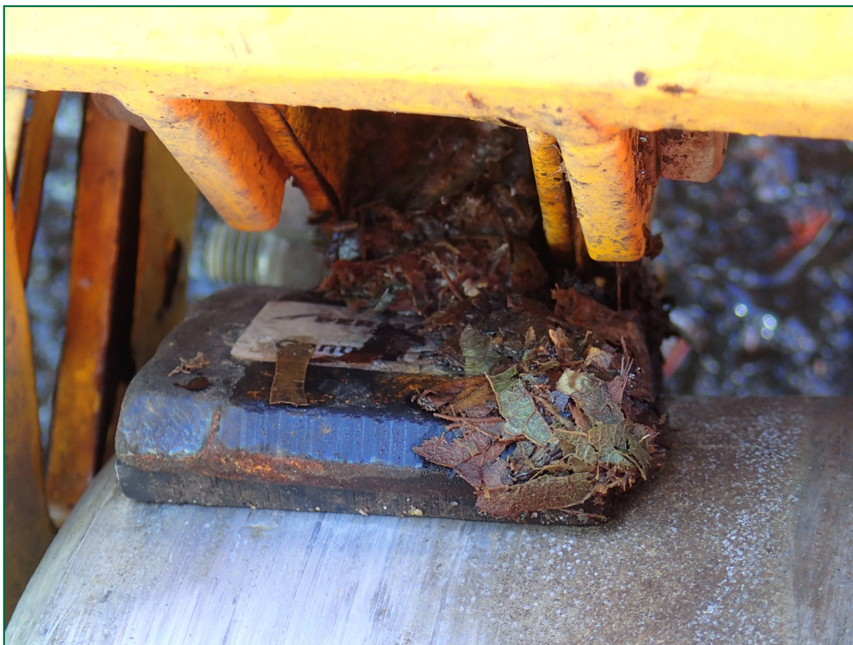
Figure 14: Leaf contamination of brake pad (ironman No. E0005087) on 3 November 2014
