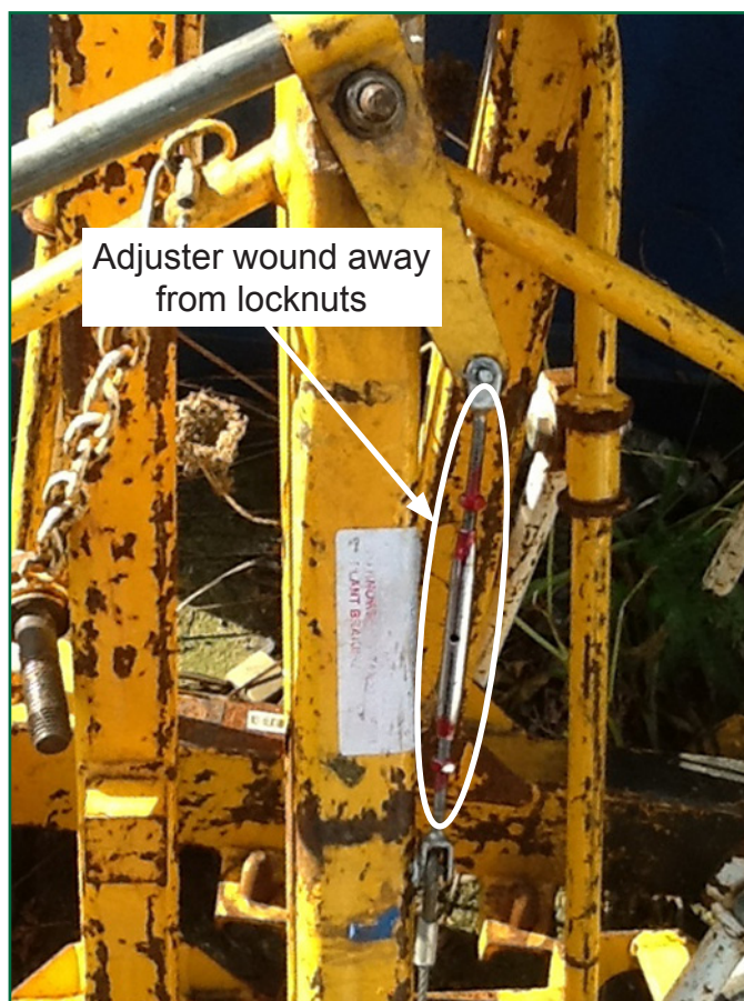
Figure 15: Evidence of interference with ironman brake adjustment (courtesy Torrent Trackside)
