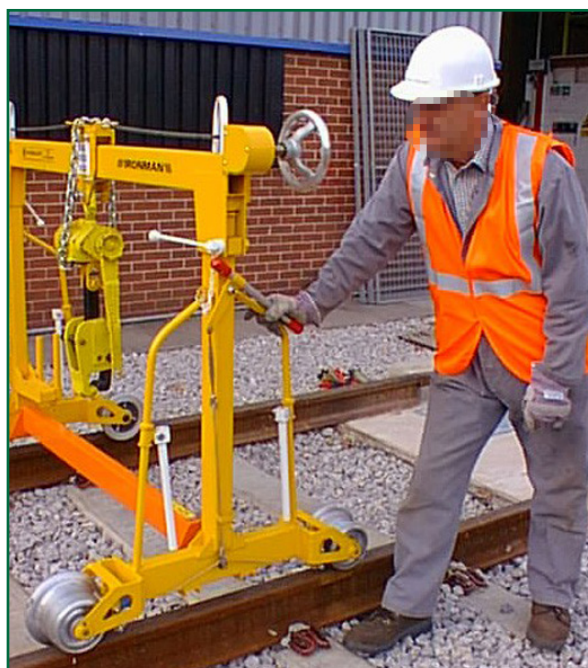
Figure 6: Use of brake handle to release ironman brakes (courtesy Permaquip)
