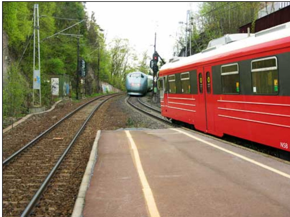
Figure 16: The trains' stopping positions after incident 2. This photo is a photomontage showing the estimated distance between the trains.
