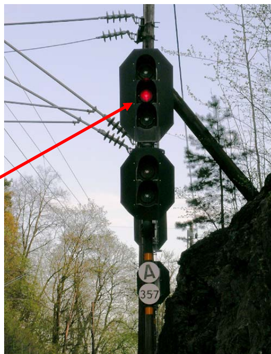
Figure 2: Block signal A Slependen was showing a "stop" signal. (Not corresponding with the signal aspect of the distant signal)
