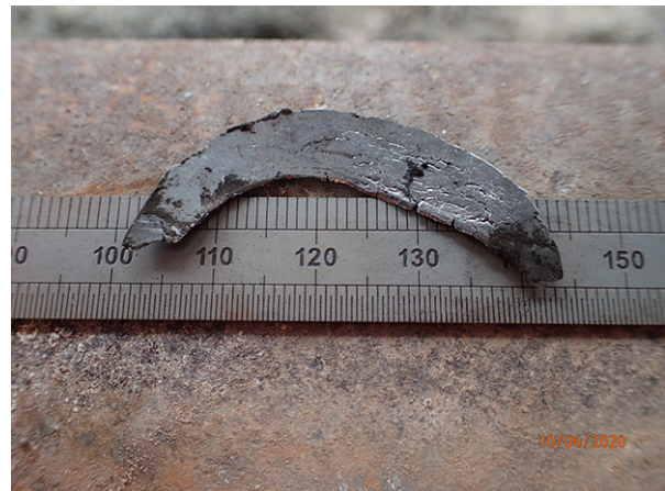
Figure 41: The largest piece of metal debris extracted from the 1-4 end top centre pivot recess
