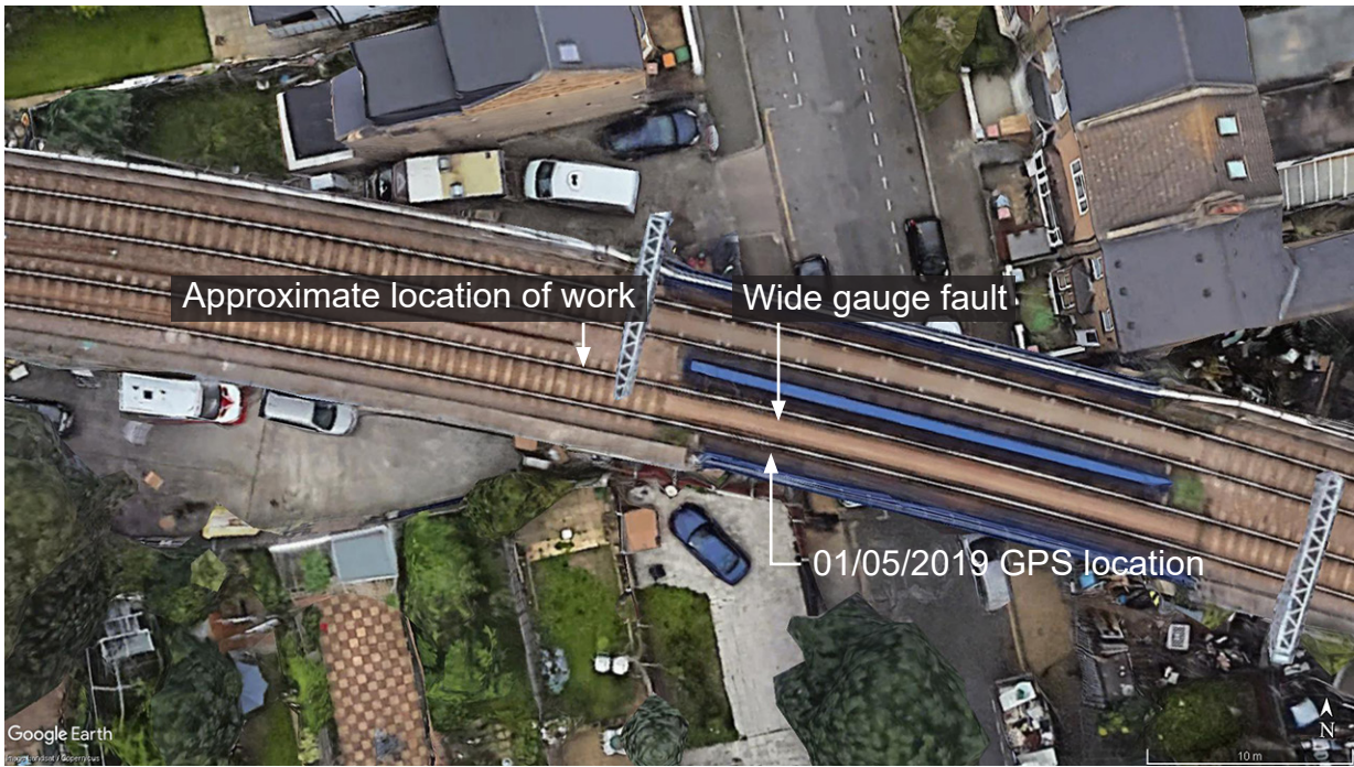
Figure 26: Google Earth image showing location of track recording vehicle-generated GPS co-ordinates and the approximate location that re-gauging work was carried out.
