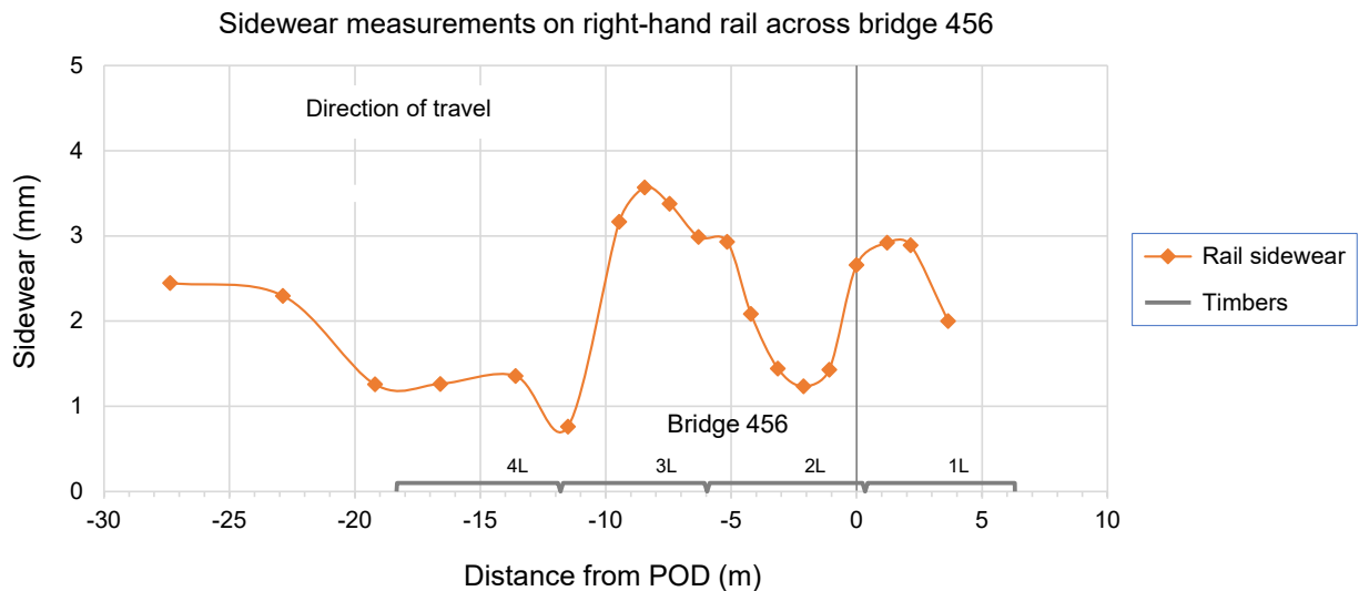
Figure 15: Change in rail wear
