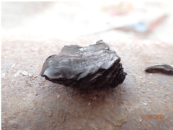
Figure 40: Part of the grease plug extracted from the 1-4 end top centre pivot recess on wagon 3415
