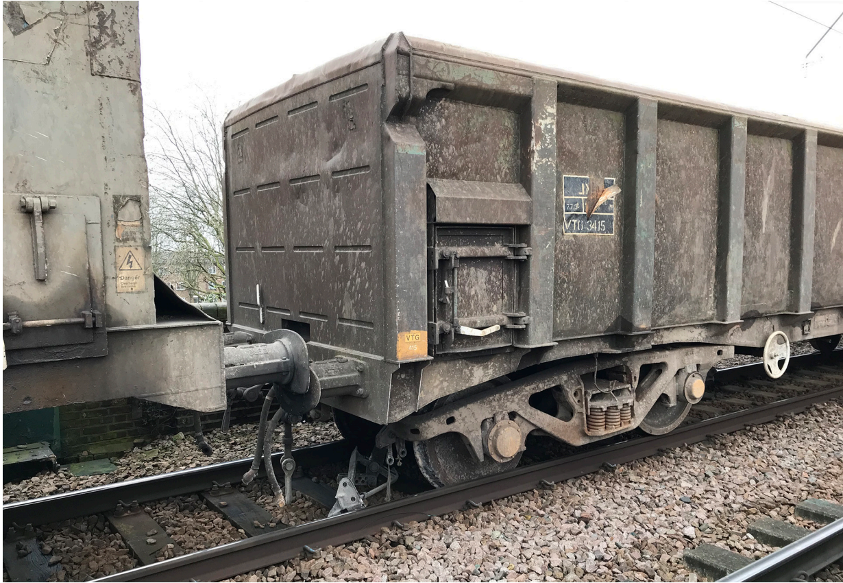
Figure 4: Wagon number 3415 with its rear wheelset derailed to the left. Part of wagon number 3114 is also visible
