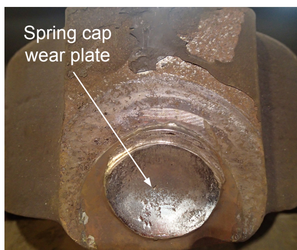
Figure 9: Wear pattern on incident spring cap wear plate
