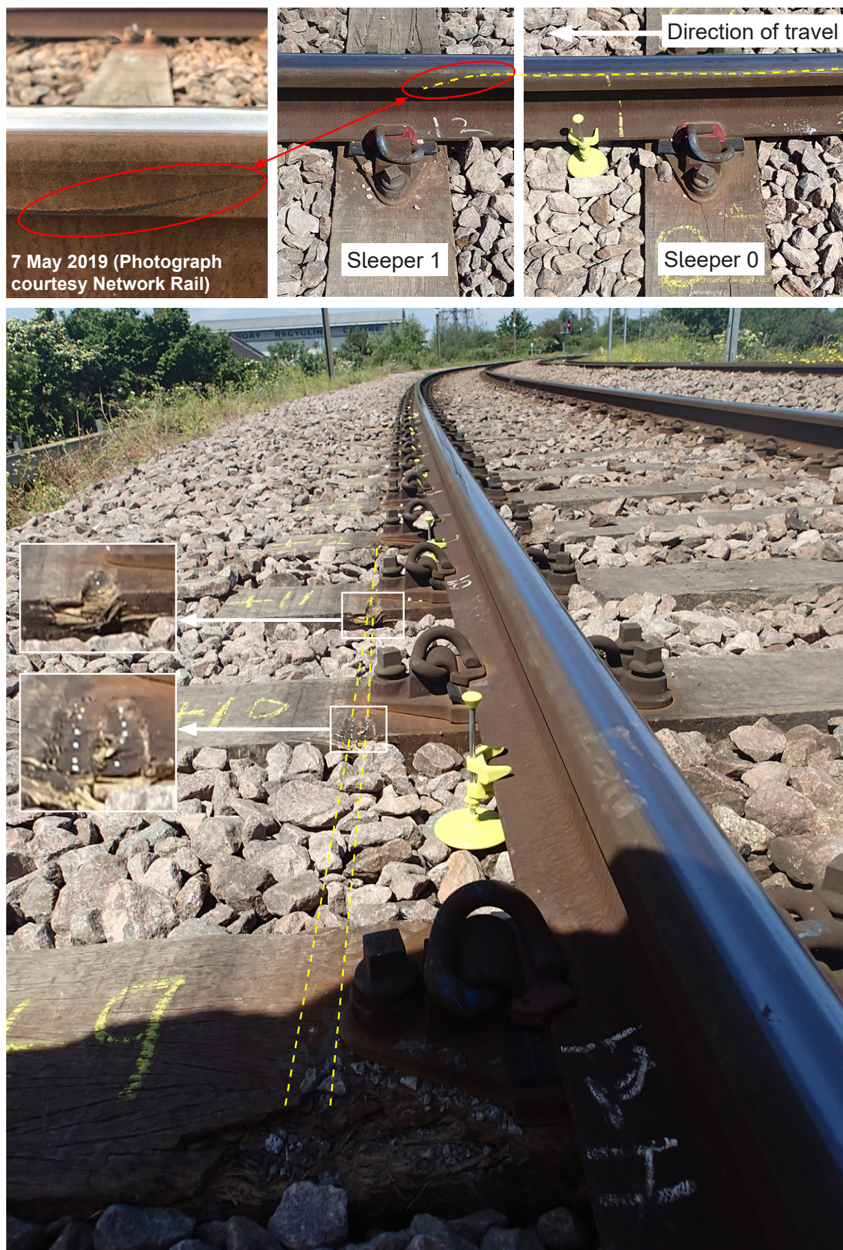
Figure 7: Marks showing evidence of derailed wheel flange running on the left-hand railhead, rail fasteners and sleeper ends (all photographs 23 May 2019, except as labelled)
