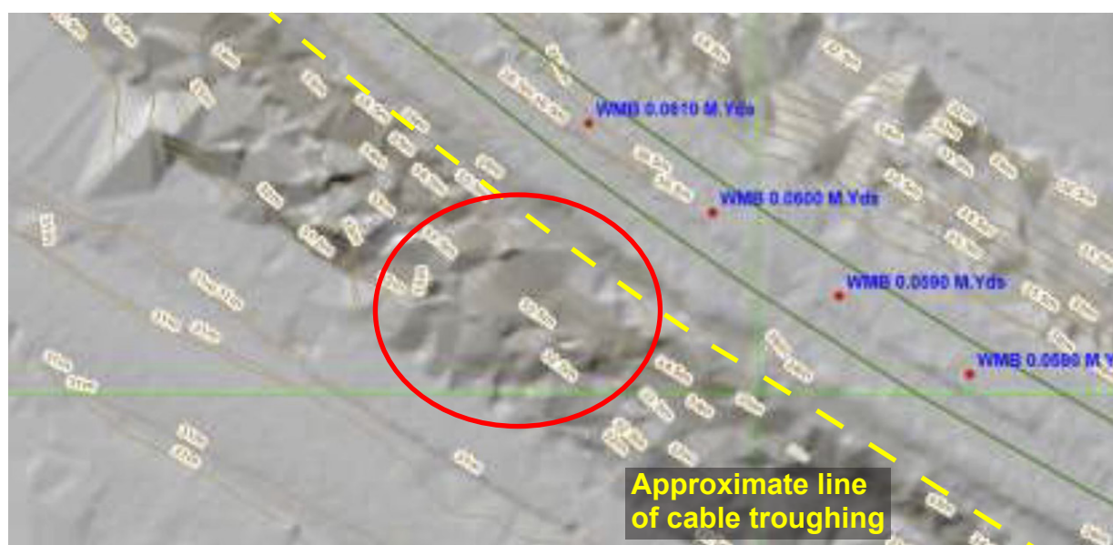
Figure 16: LiDAR survey of the embankment on Mitre Bridge Curve highlighting the flattened area on the up-side slope close to 0 miles 27 chains (image courtesy Network Rail)
