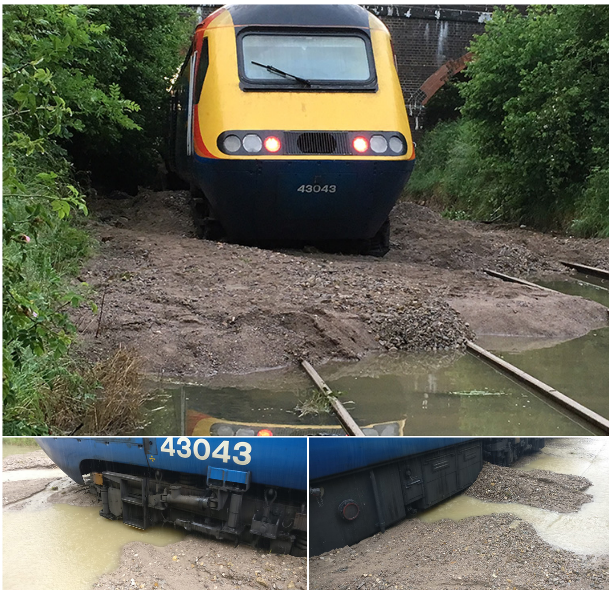
Figure 3: The rear of the train after further sandy gravel washed-out around it (main image courtesy of Network Rail, other images courtesy of the driver of train 1C52).
