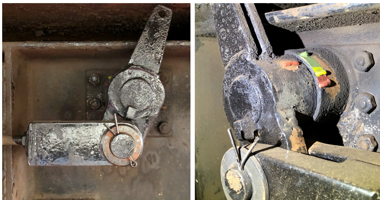
Figure 10: Photographs of the modifications made to the brake mechanism in response to the incident, showing a) the altered attachment point; and b) the tell tales used as a daily check.
