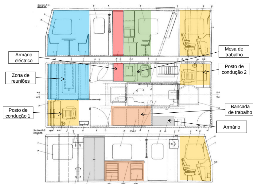
Figura 9: Diagrama interior do VCC 105 [adapt. de doc. Plasser & Theurer]
