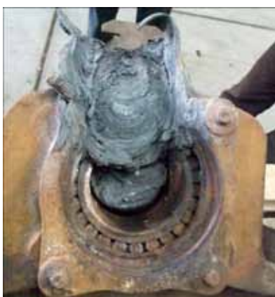
Figure 24: This photo of (the inner side of) the overheated axle box shows that the axle journal erodes its way upwards through the axle box.
