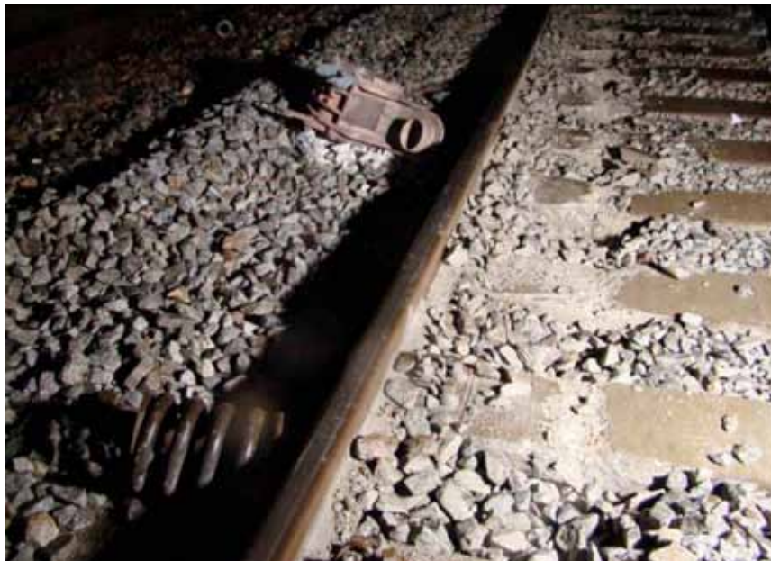
Figure 13: This photo shows the damage the left-hand wheel of the derailed wheel set caused to the concrete sleepers. The overheated axle box and one of the four springs accompanying the axle box lie next to the rail.
