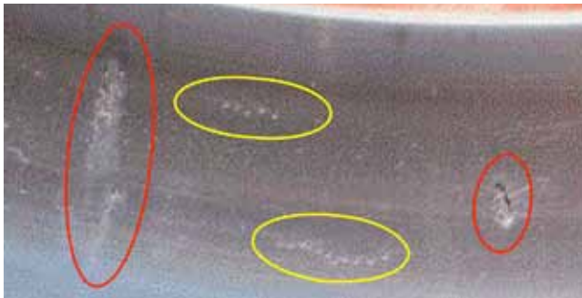
Figure 22: The adjacent photo shows the current-flow damage (circled in yellow) and chipping (circled in red) in the raceway of the outer ring of a bearing from one of the ten other axle boxes that were inspected.
