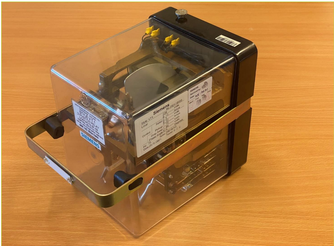
Figure 2: VT1-6F-4B relay. Photo: NSIA
