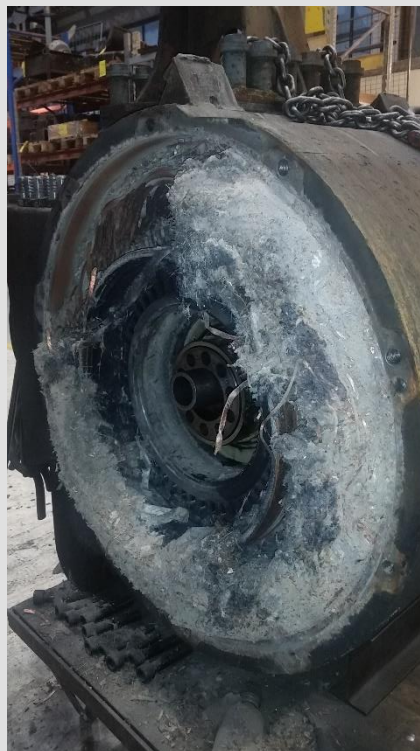
Figur 8: Demontert endedeksel. Skadet vikling. Foto: CargoNet AS
