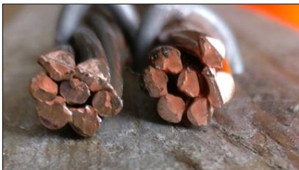
Figure 1: Cu-ETP 50/7 messenger wire cross-section.
