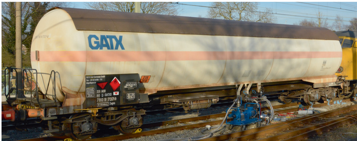
Figure 10: The damaged tank wagon was pumped empty with mobile pumps. (Photo: Dutch Safety Board)
