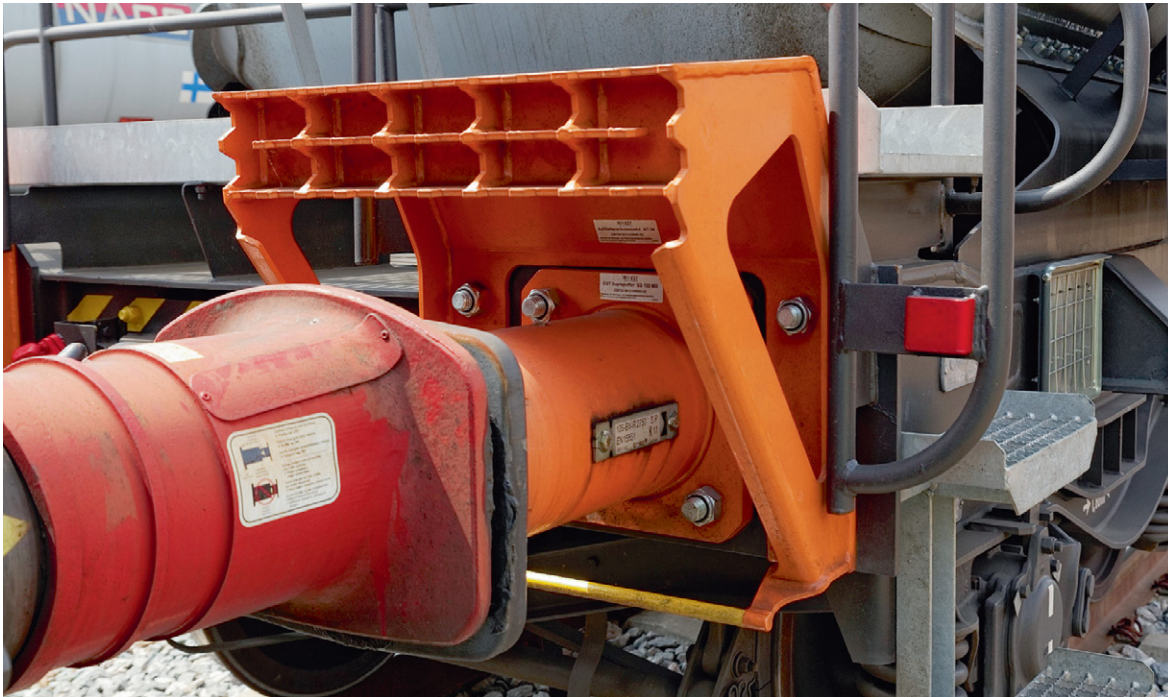
Figure 45: This photograph shows an anti climbing device. (Photo: SABIC)
