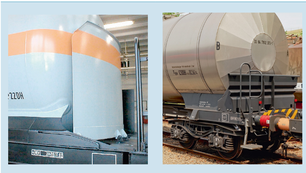
Figure 46: These photographs show two examples of protective shields. (Photos: SABIC)
