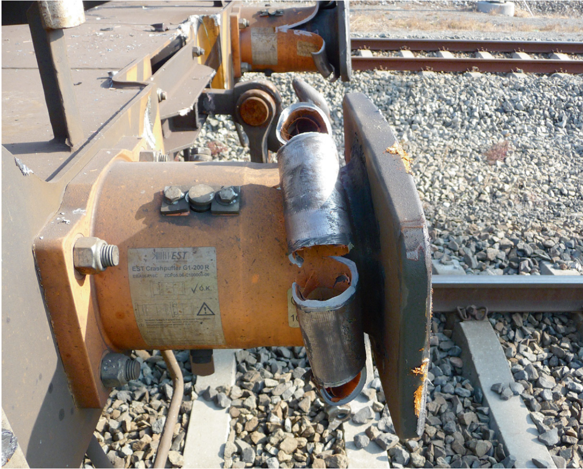
Figure 44: This photograph shows crash buffers with external absorption elements (the orange tubes) which as a result of a collision have torn and curled up, thereby absorbing energy. (Photo: Dutch Safety Board)
