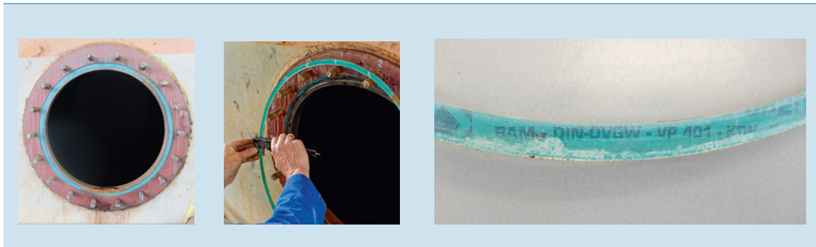
Figure 32: These photographs show the gasket. On the left-hand photograph the (green) gasket is still in the intended flange groove. On the right-hand photograph we see the markings. (Photos: Dutch Safety Board)
