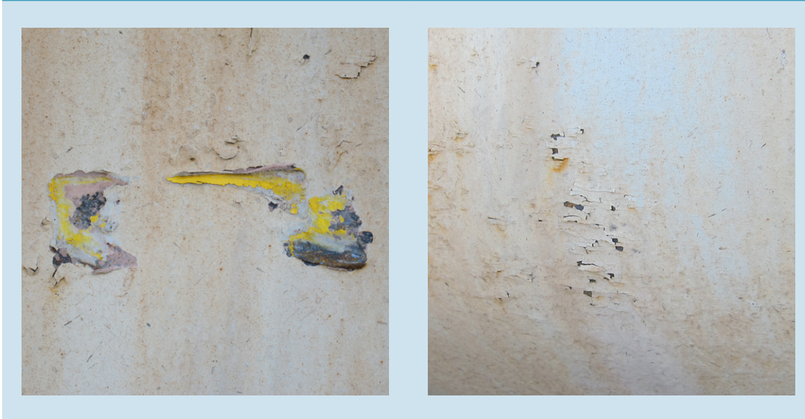
Figure 29: The left-hand photograph shows the mechanical damage observed below the manhole cover on the rear wall of the tank. The damage is the imprint of the draw eye on the front of the passenger train. The right-hand photograph shows local crackling of the paint layer on the tank. (Photos: Dutch Safety Board)
