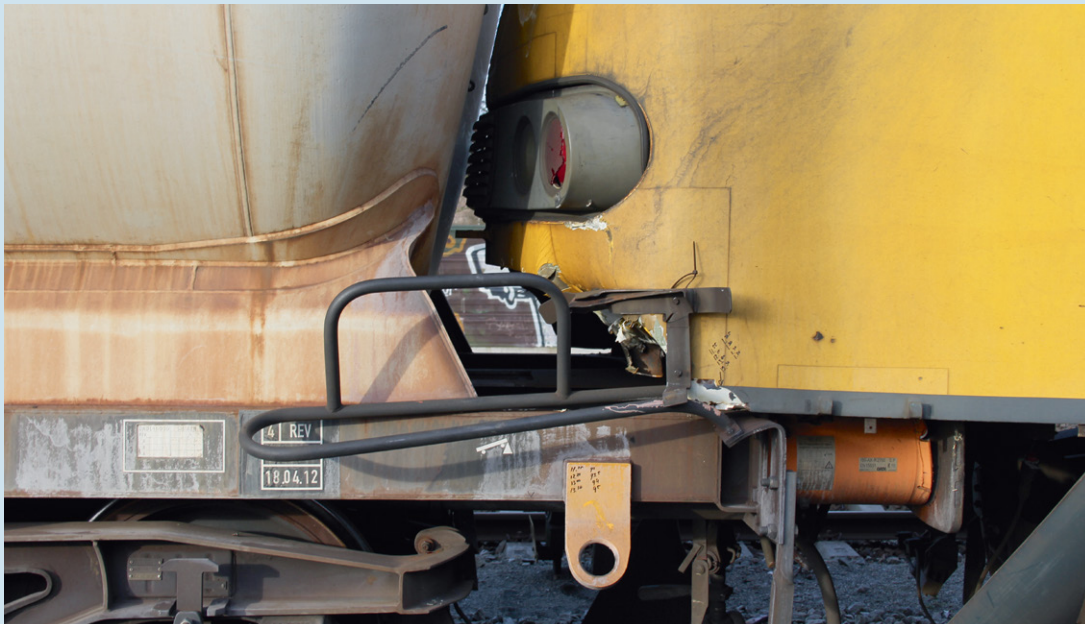
Figure 23: These photographs show that the nose of the passenger train had climbed up and over the buffers of the tank wagon, before colliding with the rear wall of the tank. (Photos: police)
