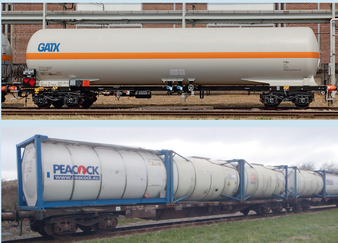
Figure 11: Examples of a tank wagon (top) and of three tank containers on a container carrier wagon (below). (Photos: SABIC)
