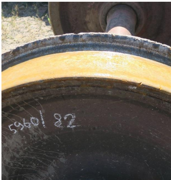
Figure 4.2.2.1: Damaged flanges of wheels 3L
