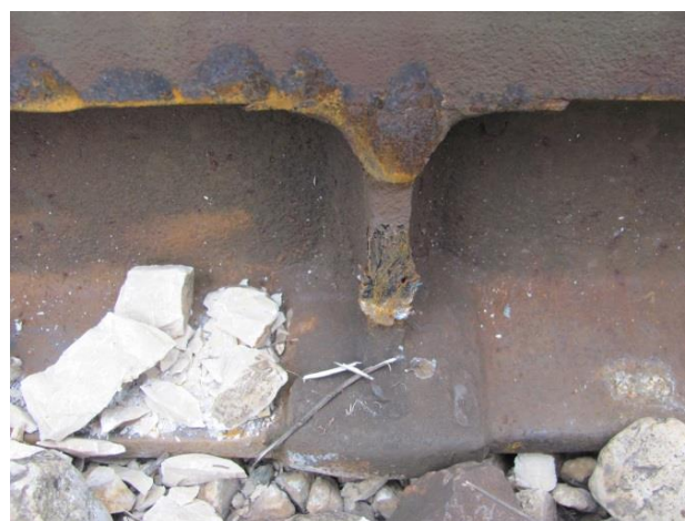
Figure 4.1.8: Trace of the second impact of the left fallen wheel on the welded joint
