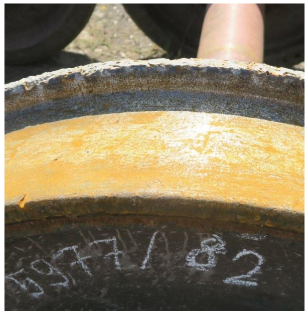
Figure 4.2.2.2: Damaged flanges of wheels 4L
