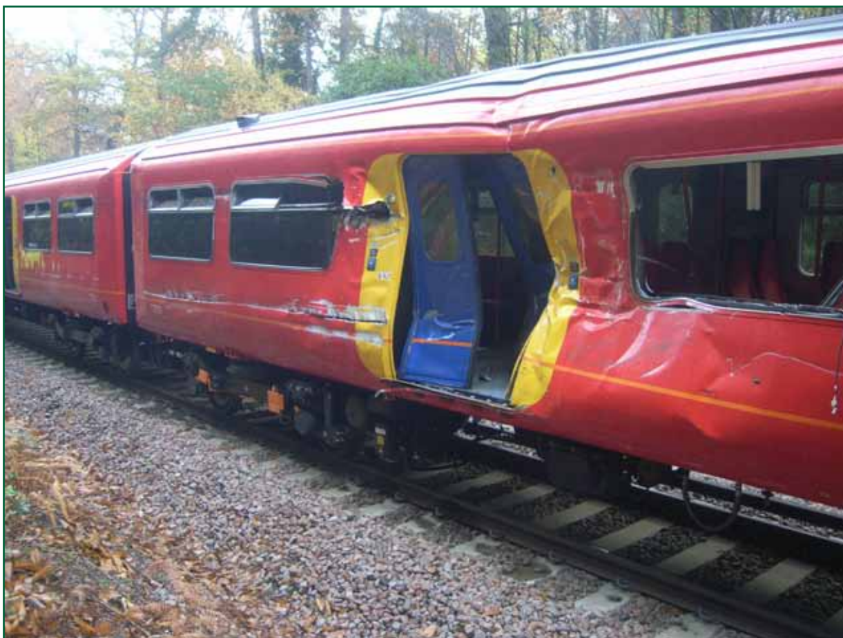
Figure 8: View of coach 8 which sustained a side impact from the disintegrating lorry chassis
