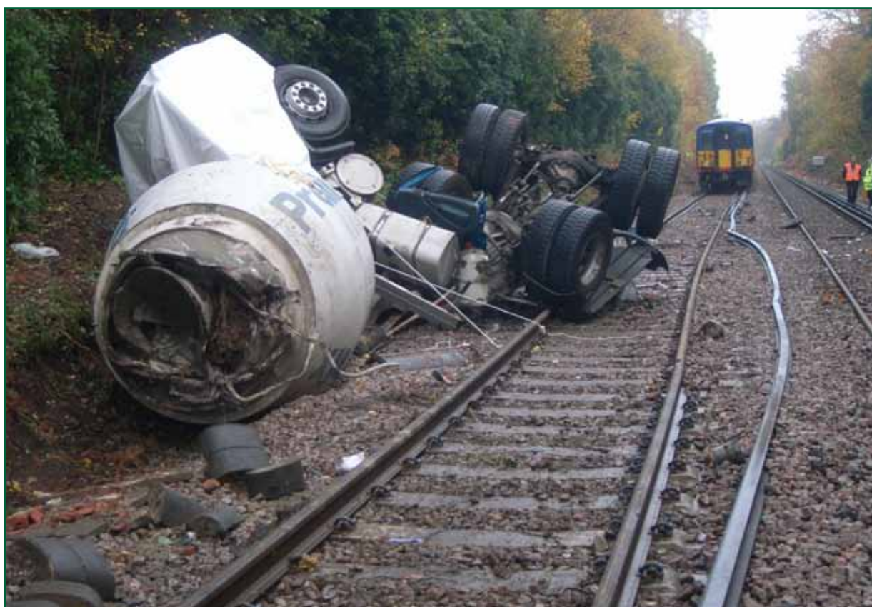
Figure 9: View of damaged lorry and train. Note displaced track and conductor rail
