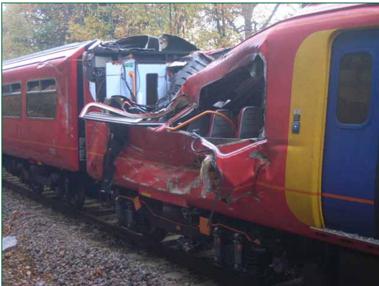
Figure 7: View of coach 6 (leading end) which sustained a vertical impact from the falling lorry
