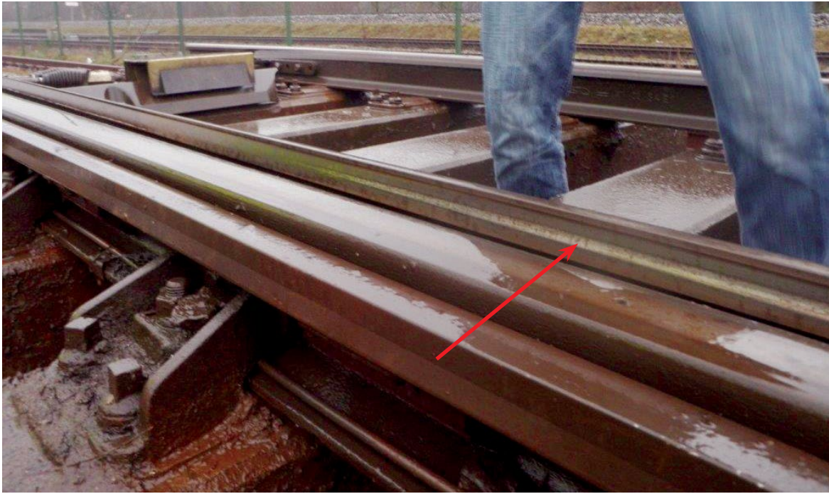
Figure 8: Flange-back contact marks on the right-hand switch blade of switch 3B. (Source: ProRail)
