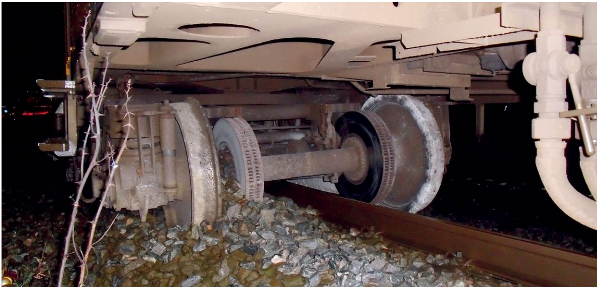
Figure 3: Wheel set of the second carriage that ended up alongside the rails. (Source: upper photograph Nedtrain, lower photograph ProRail)
