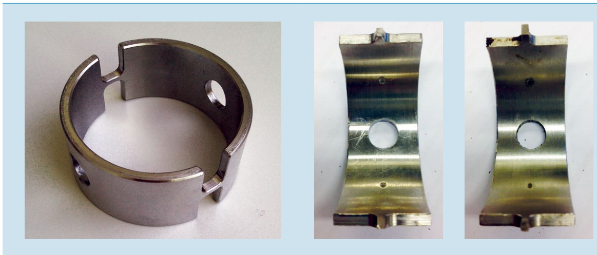
Figure 28: The photograph on the left shows an undamaged ring. The two photographs on the right show the ring from switch 3B, broken into two halves. (Source: ProRail)
