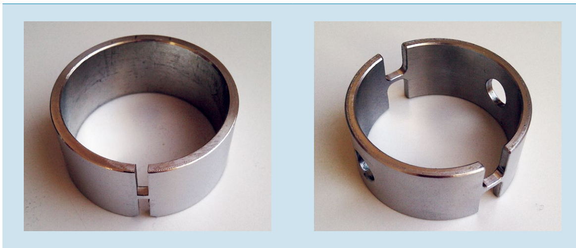
Figure 38: The left-hand photograph shows a ring of the original type (with a single break link and square corners); the right-hand photograph shows the modified version (with two break links and rounded corners). (Source: ProRail)
