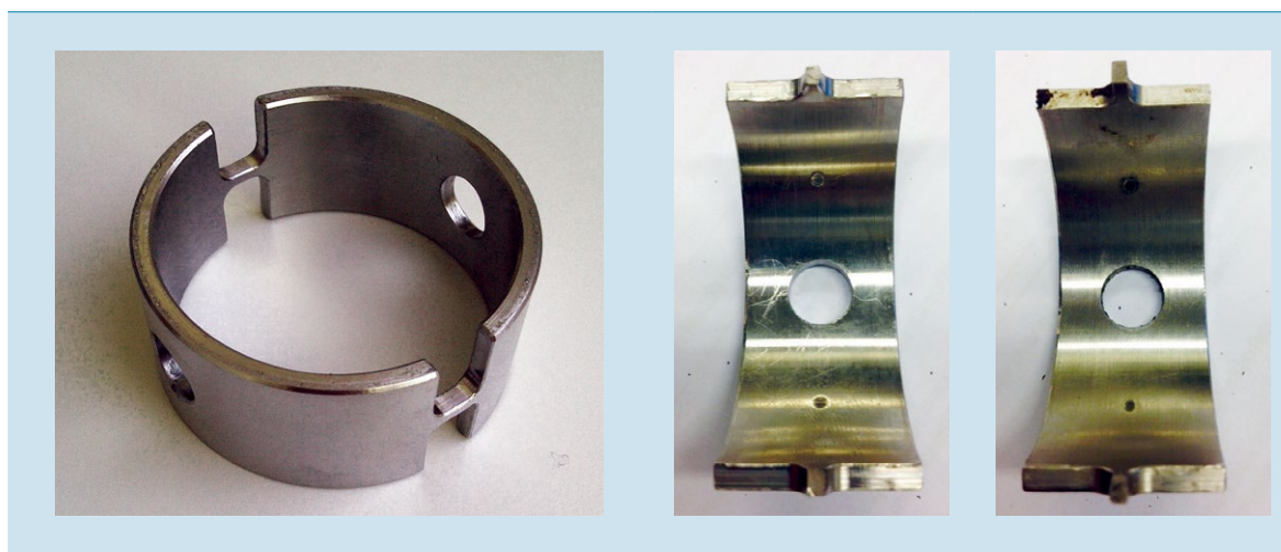
Figure 6: Ring: left an intact example; on the right, the two broken halves of the ring from switch 3B in Hilversum. (Source: ProRail)
