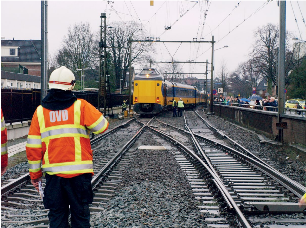
Figure 25 The photograph shows the final situation (seen in the direction of travel of the train). In the foreground, the first crossover switch is visible, with in the background, the rear section of the train. (Source: Jan Barnier – Model Centre Hilversum)
