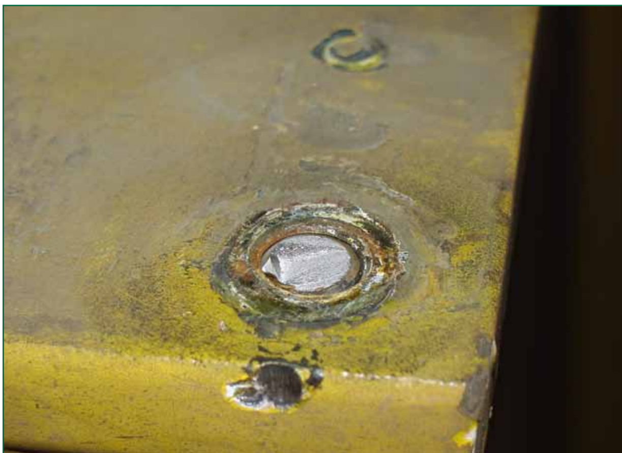
Figure 11: Lower section of bolt R4 (inserted into cab roof) showing clean-break indicating overload failure of the bolt
