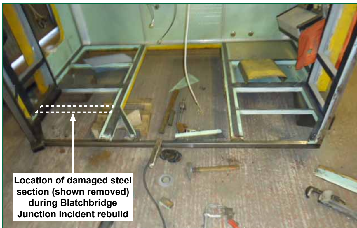
Figure 23: Damaged steel section removed for replacement during re-build of the P3 cab after the incident at Blatchbridge Junction. The front of the cab is lying face down in this image.
