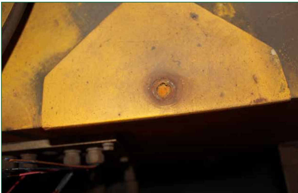
Figure 10: Lower section of bolt F2 (inserted into cab roof) showing rusted-over fracture face
