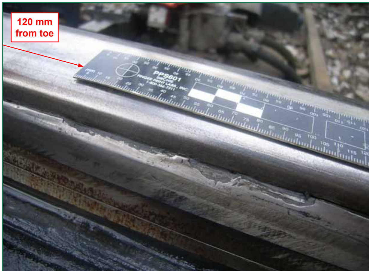
Figure 7: Left-hand switch rail damage
