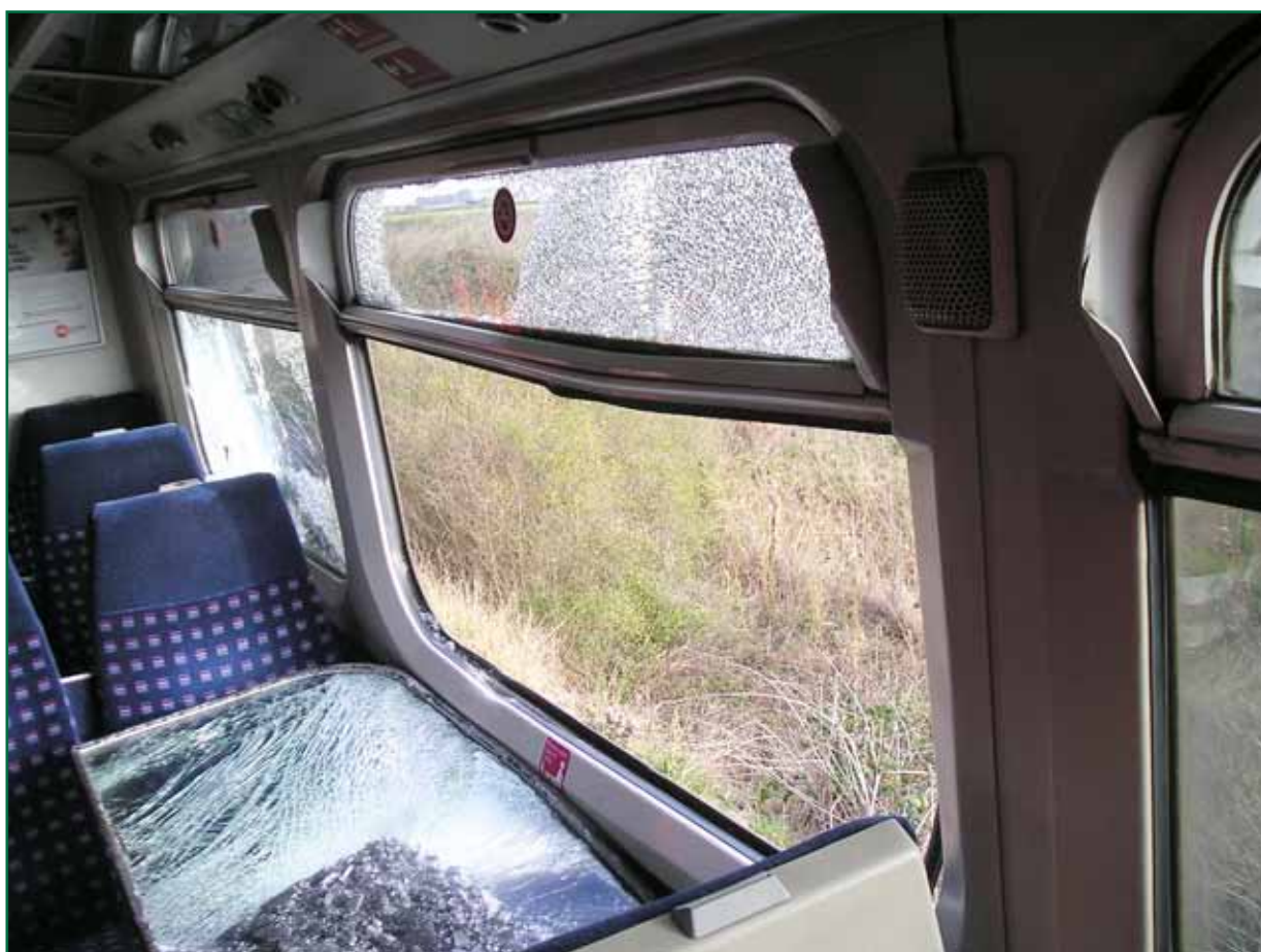
Figure 7: Window after falling into passenger area (courtesy of First Capital Connect)
