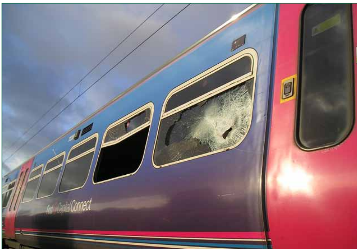
Figure 6: External damage to the train (courtesy of First Capital Connect)
