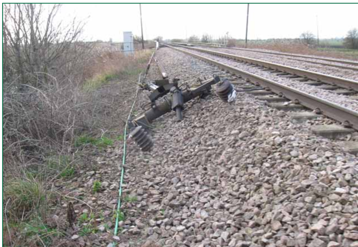
Figure 5: Remains of the pantograph in the cess (courtesy of Network Rail)
