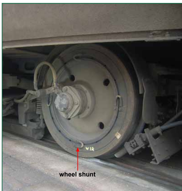
Figure 13: Leading bogie of tram 2538 showing wheel shunt
