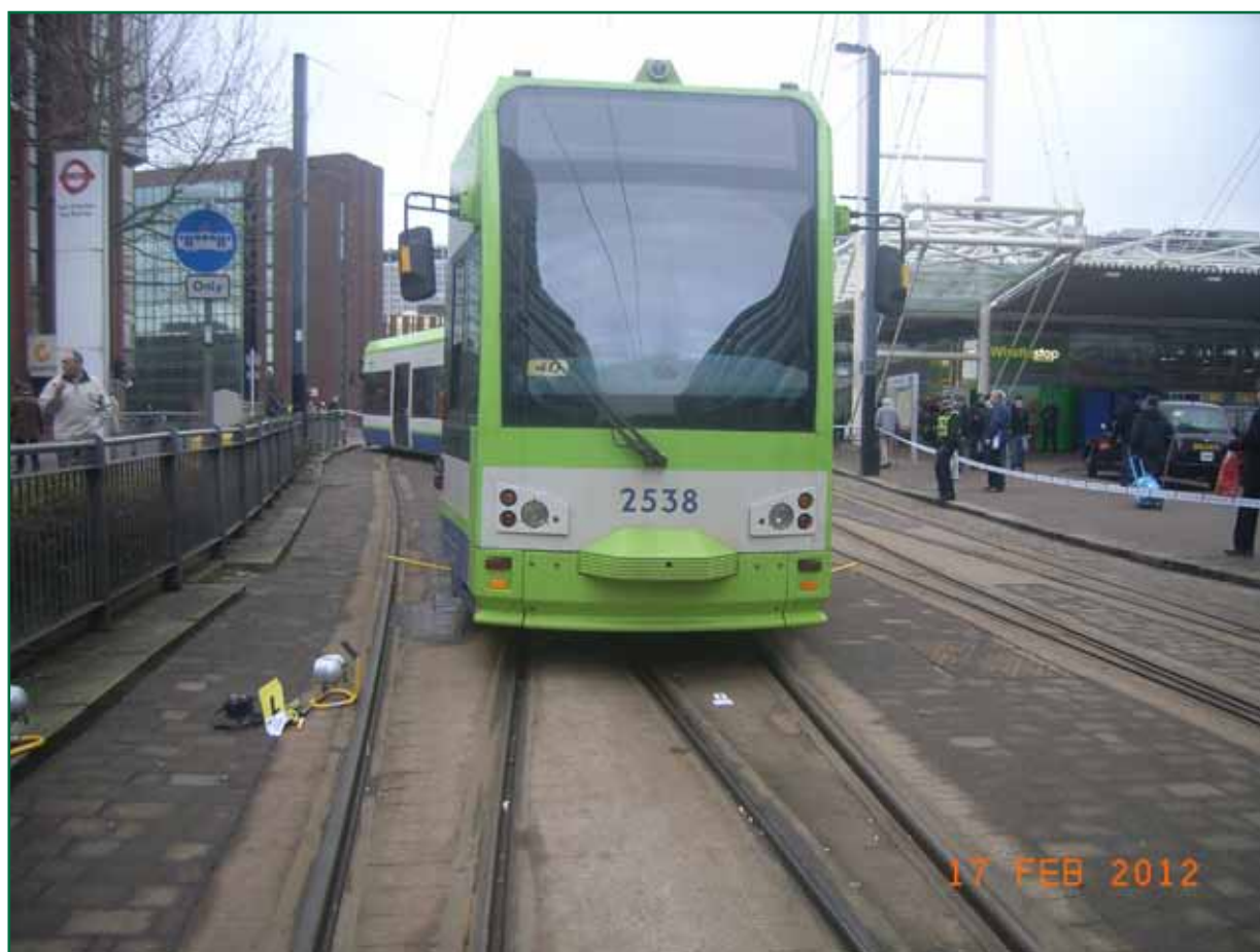
Figure 7: Rear view of tram 2538 following derailment
