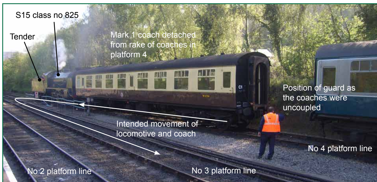
Figure 2: The accident site at Grosmont station showing a reconstruction by the RAIB of the accident circumstances
