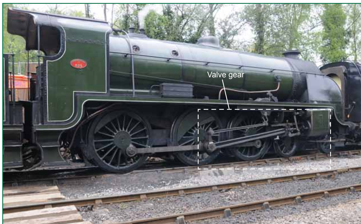
Figure 5: Valve gear fitted to S15 class locomotive no.825 with the locomotive in reverse gear
