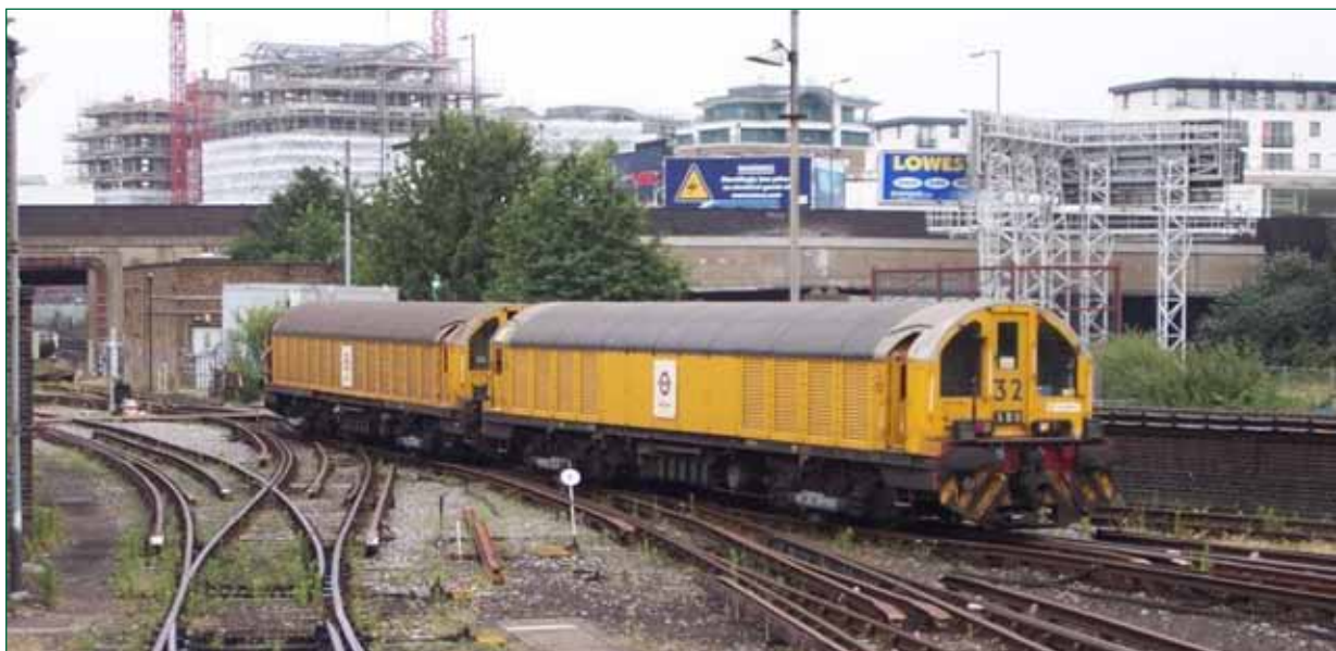
Figure 5: Two battery locomotives (image courtesy of Tube Lines).
