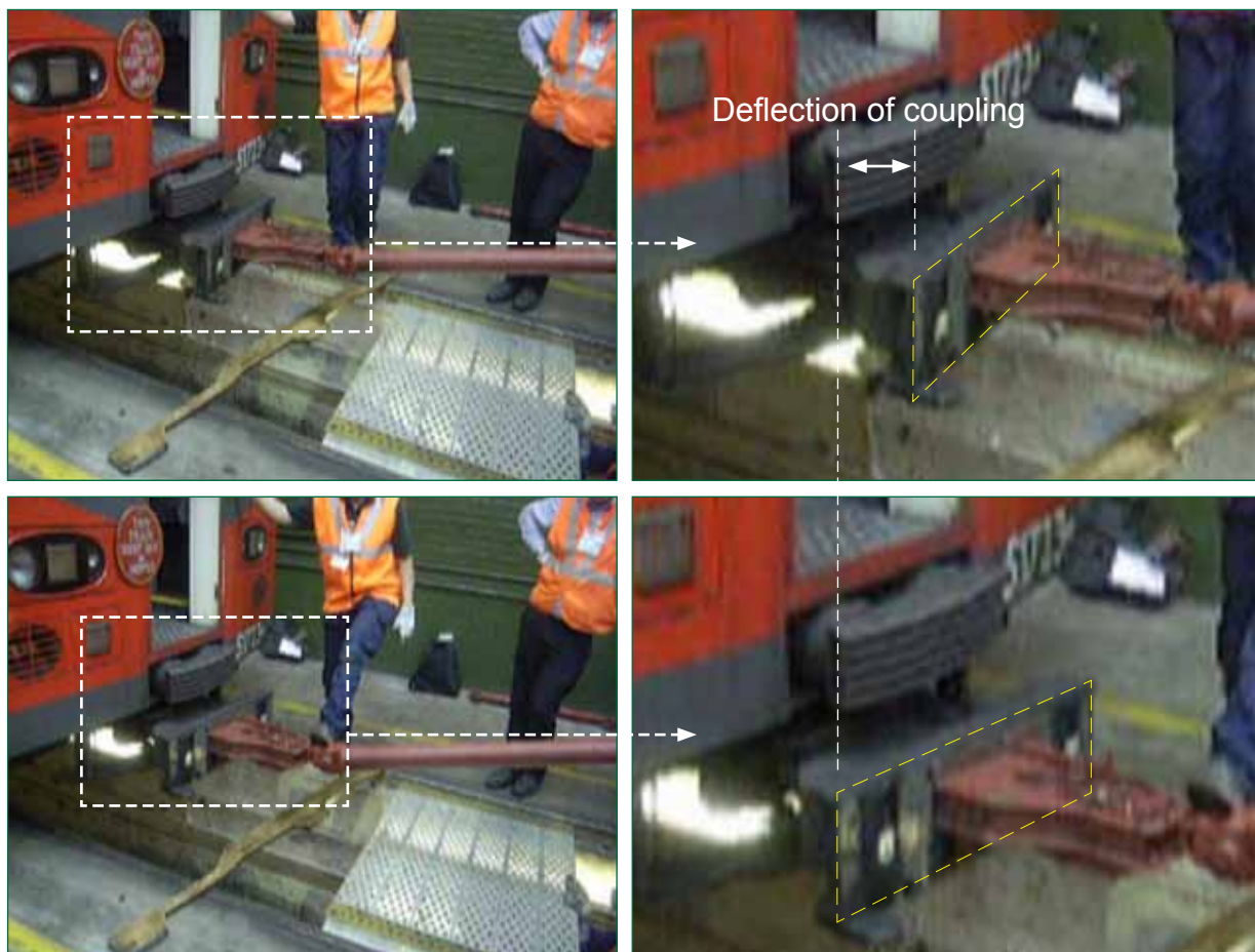
Figure 16: Lateral coupling deflection observed during post-incident RAIB testing.
