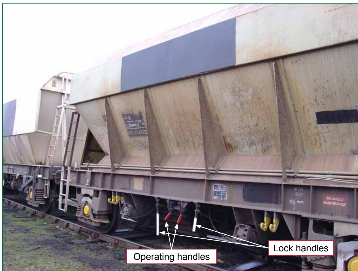
Figure 4: Wagon 14513, showing door control and locking handles
