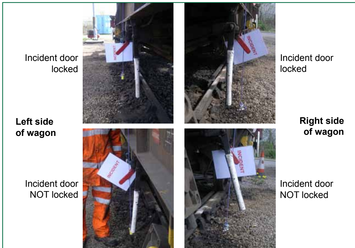
Figure 8: Variations in handle position between doors locked and unlocked
