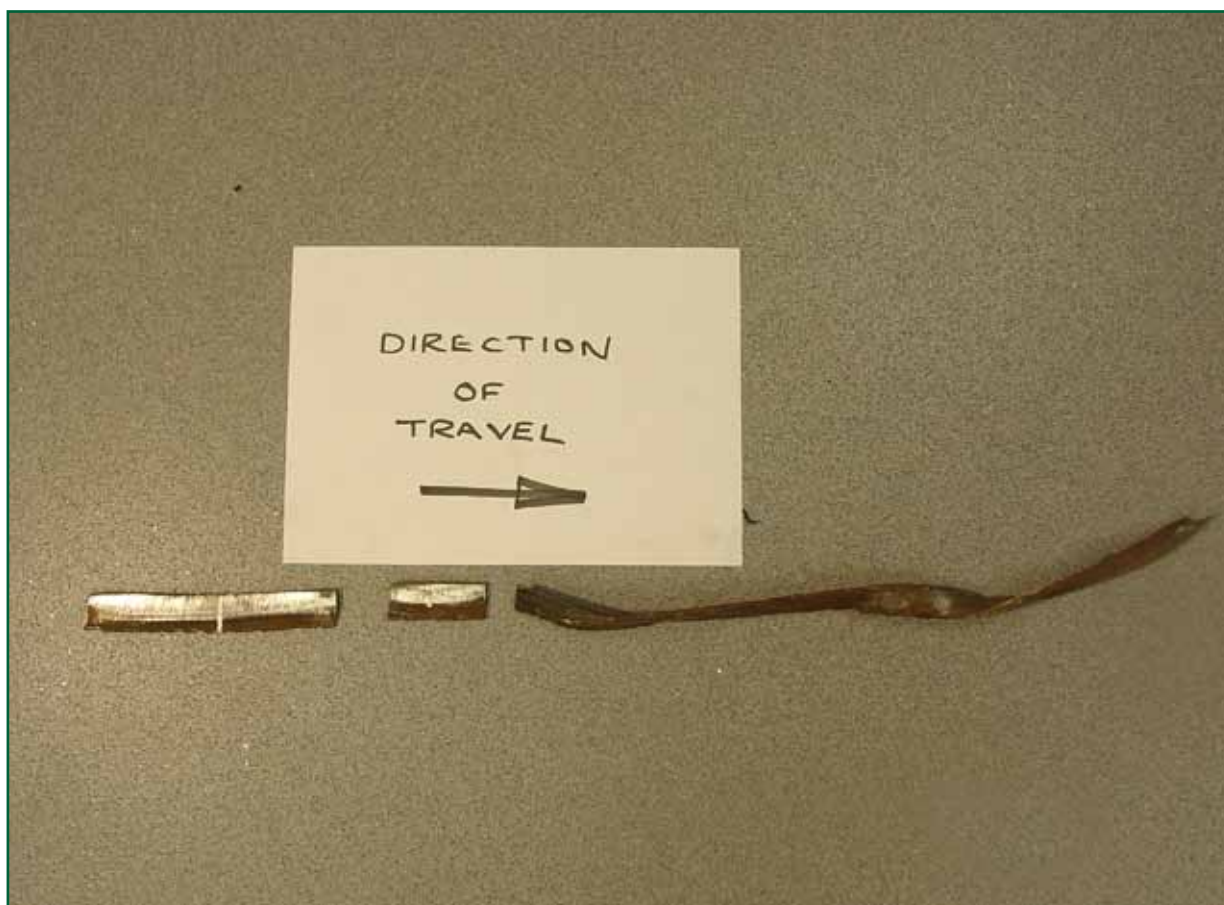
Figure 5: The failed section of the keep
