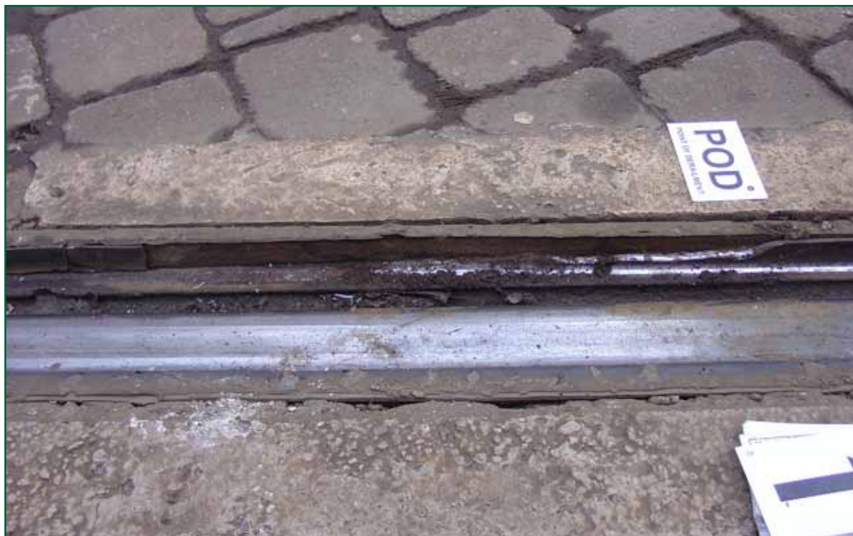
Figure 4: The right-hand rail at the point of derailment where the keep had failed
