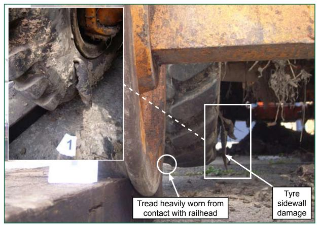
Figure 12: A rail wheel and its adjacent treaded tyre
