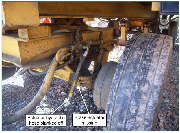
Figure 16: Defective brake on the leading wagon
