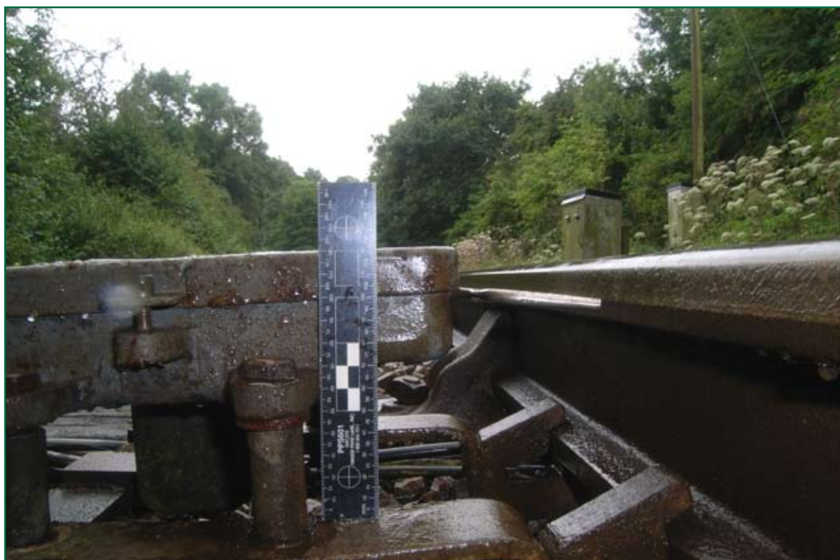
Figure 14: Displaced treadle arm
