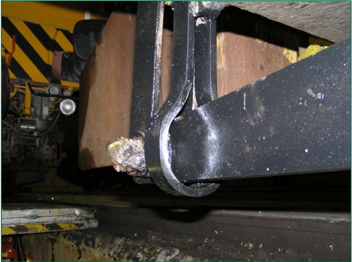
Figure 19: USP 3000 ballast regulator torque arm with recommended safety keep. Similar safety keeps have been fitted to all NIR OTP
