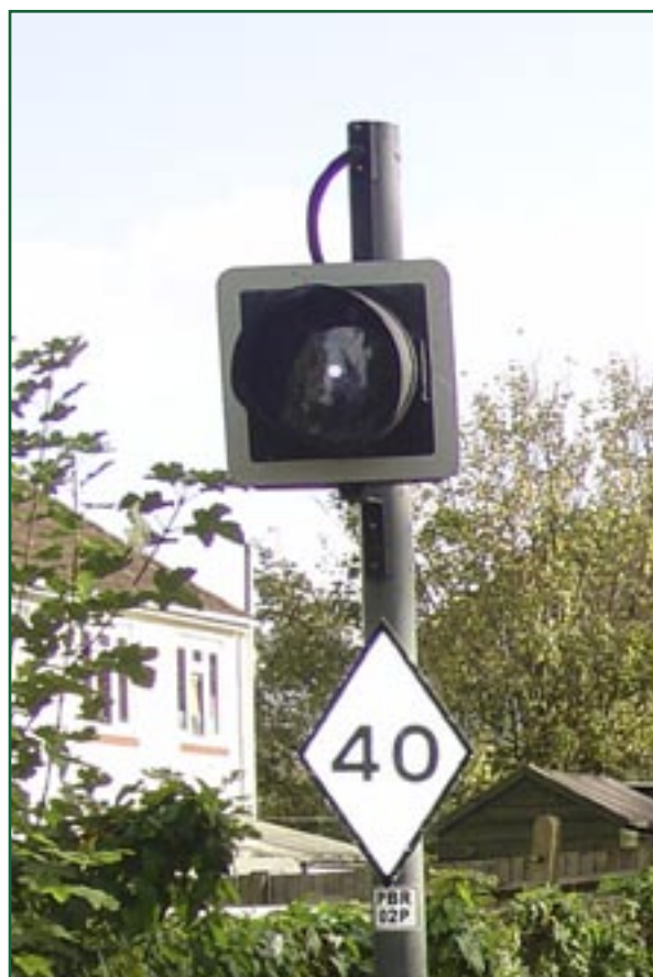
Figure 3: Points position indicator - points not correctly set
