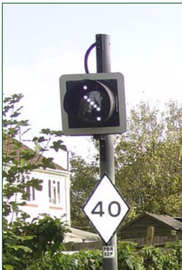
Figure 2 : Points position indicator - points correctly set
