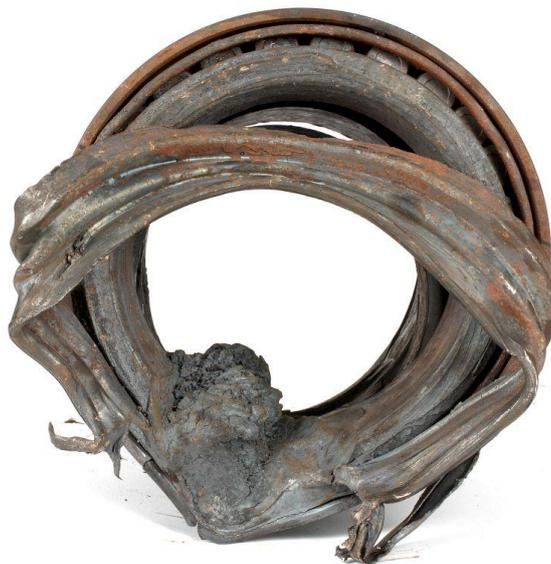
Photo 3 – Failed Bearing
