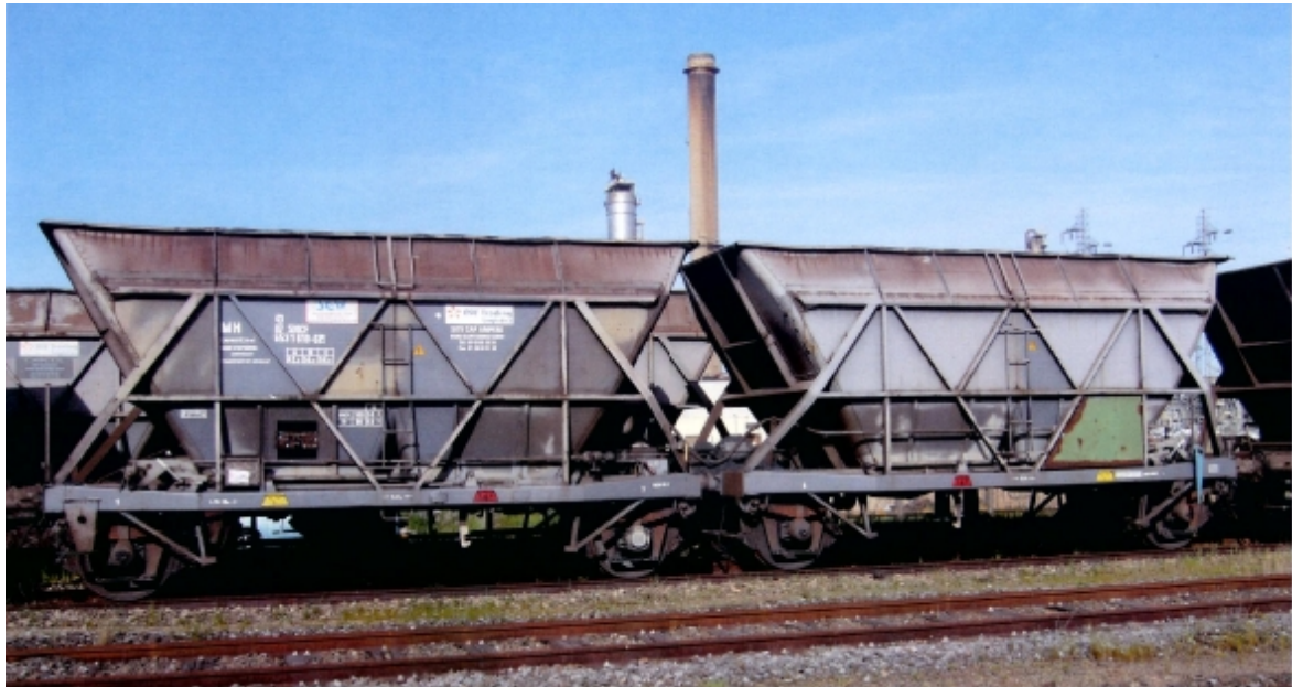
Illustration 5 : Wagon trémie EFc60
