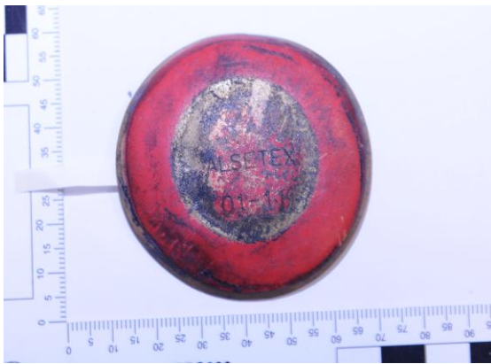
Figure 20 – Fog signal that was found at the bottom of the tube
