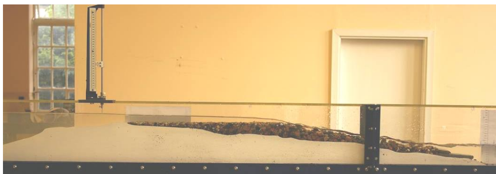
Photograph 6 – 2-D model in laboratory flume
