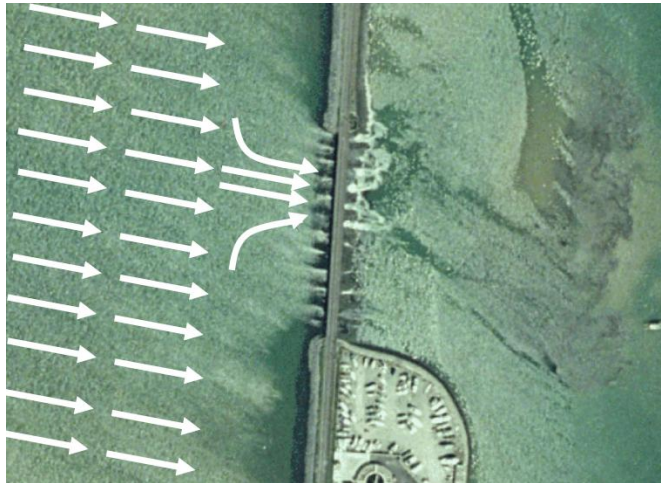
Photograph 10 – Majority of water flow between Piers 4 and 5
