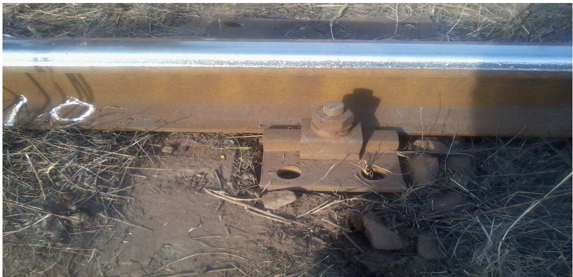
Photo 1. The place where the climbing of the right wheel flange, in the running direction, on the head of rail, corresponding to the exterior curve rail happened.
