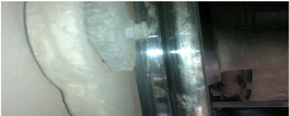
Photo 2 Scoring existing on the axle no. 1, derailed wheel
