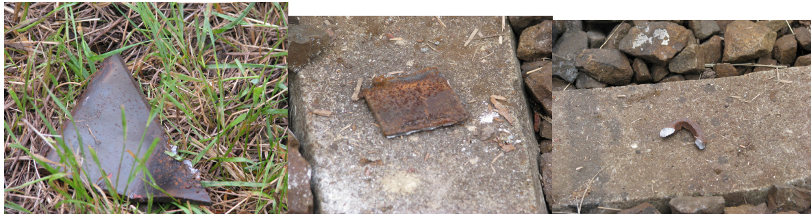
Picture 4 - metallic pieces detached from the derailed wagon and the fallen clack
