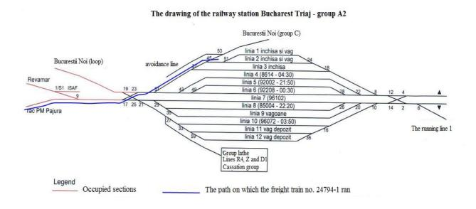
The drawing of the derailment after the accident on the switch 45 railway station Bucharest Triaj, Station 17, on the 19<sup>th</sup> of January 2011
