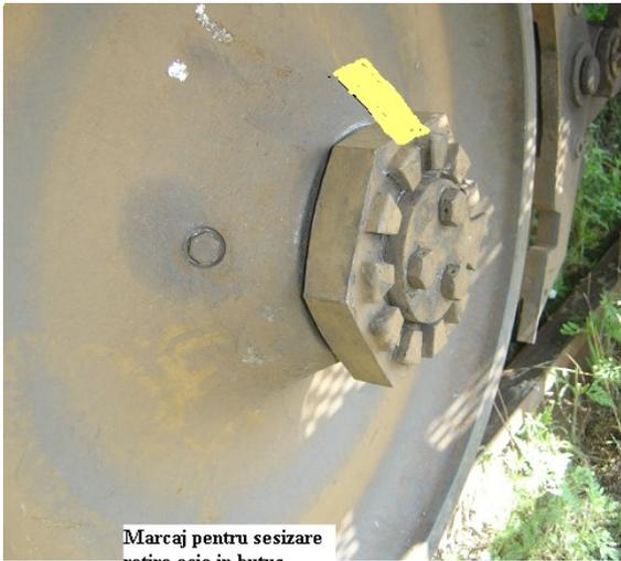
Following this railway accident, SC KRON – TRIEM SRL Braşov and SC Regiotrans SRL Braşov management teams ordered, for this rolling stock, to be marked with paint to highlight the axle spins in the wheel boss.
