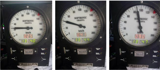
Taking into account that the real value of the wheel diameter (1241 mm) is smaller than the value of the maximum wheel diameter (1250 mm), introduced as reference element in the memory of the ITSMR equipment, results that the real speed of the locomotive was under that registered in the memory of the ITSMR equipment of the locomotive.
